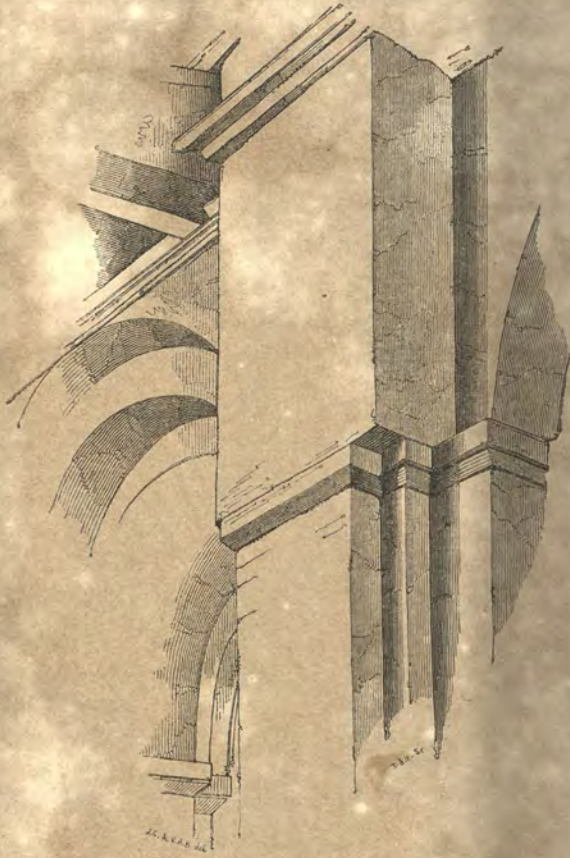
Pilaster-buttresses of the clerestory, as seen in the North aisle of the Choir.
