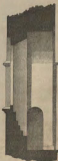
Section of the clerestory wall.
