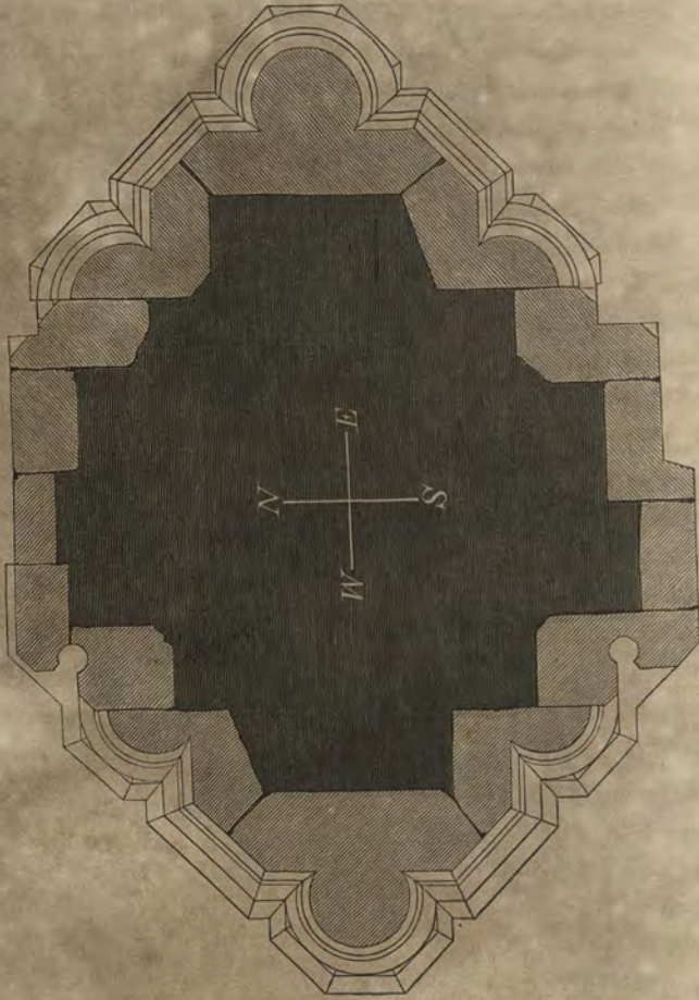
Plan of the Norman pier on the South side of the Nave, with the ashlaring of William de Trumpington and Roger de Norton.
