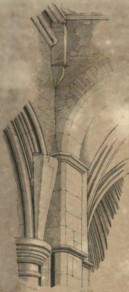
The Norman pier on the South side of the Nave, with the ashlaring of William de Trumpington, and Roger de Norton, as seen in the aisle.
