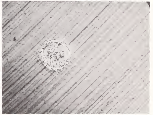
Figure 3. Nomarski micrographs of damage sites showing cratering on a diamond-machined electroplated gold surface with the initial sample temperature at 139°K in (a) and 276°K in (b). No differences in morphology are evident.
