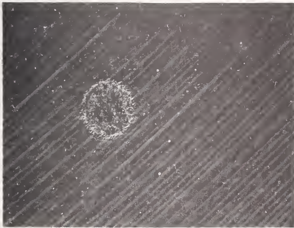
Figure 3. Nomarski micrographs of damage sites showing cratering on a diamond-machined electroplated gold surface with the initial sample temperature at 139°K in (a) and 276°K in (b). No differences in morphology are evident.
