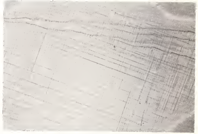
Figure 6. Surface damage on LiF, 100 shots, fluence 1.7Jcm -2 .
