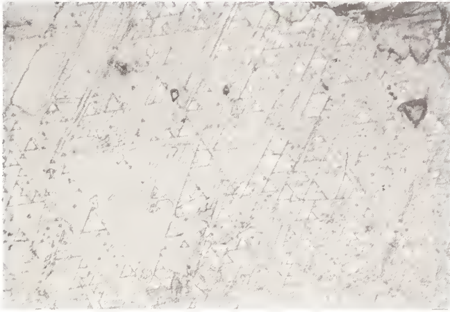
Figure 5. Surface damage on SrF 2 , 1 shot, fluence 4.2Jcm -2 .
