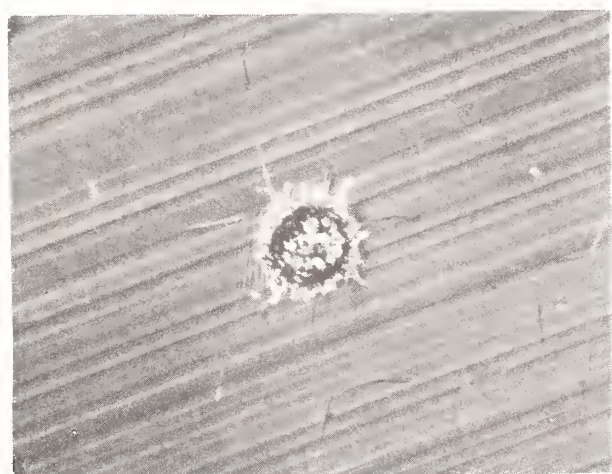
Figure 1. Nomarski micrographs of damage sites showing cratering on a diamond-machined OFHC copper surface with the initial sample temperature at 133°K in (a) and 300°K in (b). No differences in morphology are evident.
