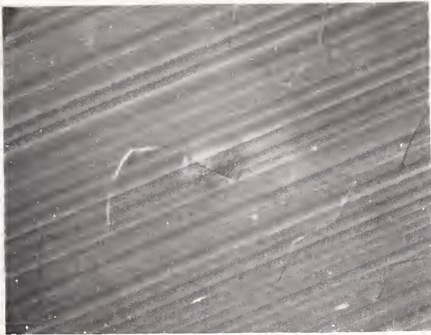
Figure 2. Nomarski micrographs of damage sites showing slip on a diamond-machined OFHC copper surface with the initial sample temperature at 133°K in (a) and 300°K in (b). No differences in morphology are evident.
