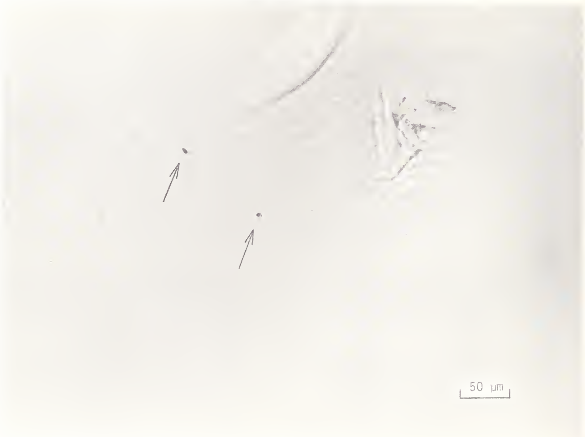
Figure 10. Nomarski micrograph of laser damaged site on the fused silica sample polished by VTI, Inc., taken with Nikon Optiphot (Two arrows indicate pits after 5 minutes etching with 5 % HF).
