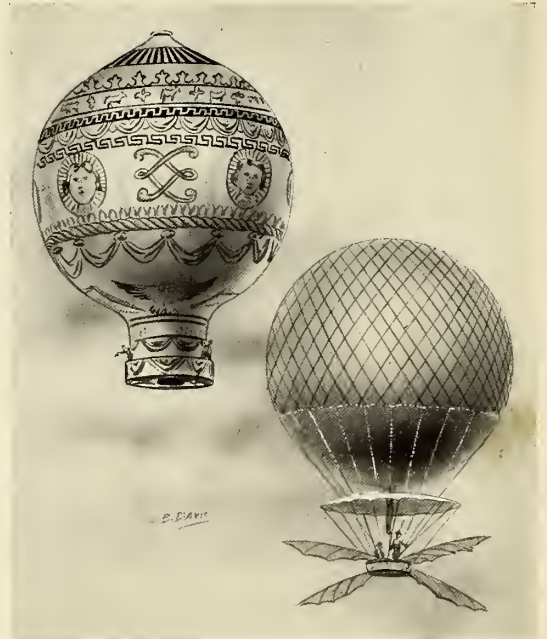
THE GAUDILY DECORATED BALLOON OF THE MONTGOLFIER BROTHERS AND THE ONE USED BY BLANCHARD. Note the parachute on this one as a safeguard in case of the collapse of the balloon; also the wings for protection.
