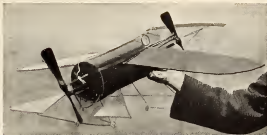
FIG. 14. A CYLINDRICAL MODEL WHICH FLIES WELL.
