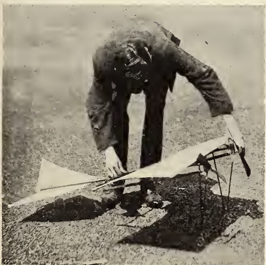
ELEVATING THE FRONT PLANE.
