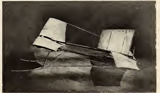
FIG. 3. HERE THE VERTICAL RUDDER IS TOO LARGE—OTHERWISE IT IS AN EFFICIENT MODEL.
