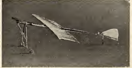
FIG. 2. A SIMPLE MODEL. THE PROPELLER AT THE LEFT, WHICH IS THE FRONT, EXTENDS TOO FAR BEYOND THE FRONT PLANE.
