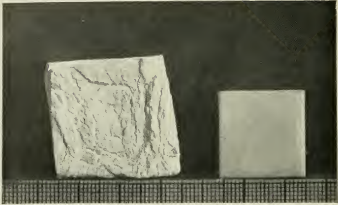
(a) Cube of Carrara marble before and after deformation
