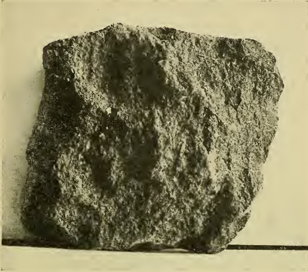
FIG. 4.—The common type of diabase showing hackly fracture. About one-half natural size.
