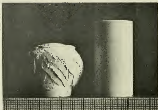
(b) Column of Carrara marble before and after deformation, using alum as an embedding material
