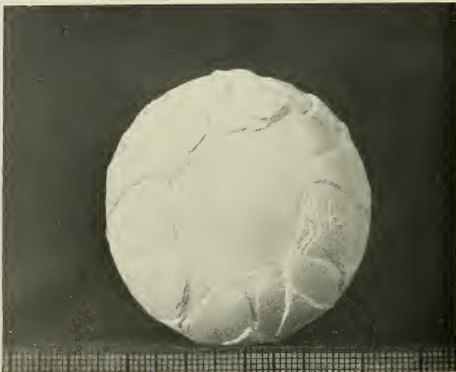
(c) Sphere of Carrara marble after deformation
