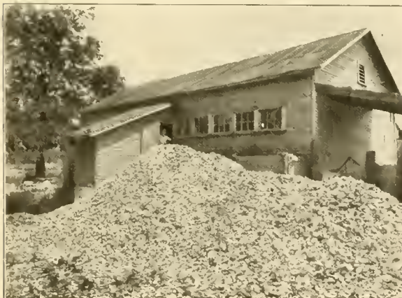
FIG. 41. A button factory at Devall Bluff. Observe the huge pile of shells in the foreground out of which buttons have been cut.
