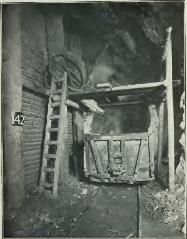
Fig. XII—Photograph of Mine Chute. A wooden, gable-bottom car is shown in the figure. This is used specially for sill floor shovelling.
