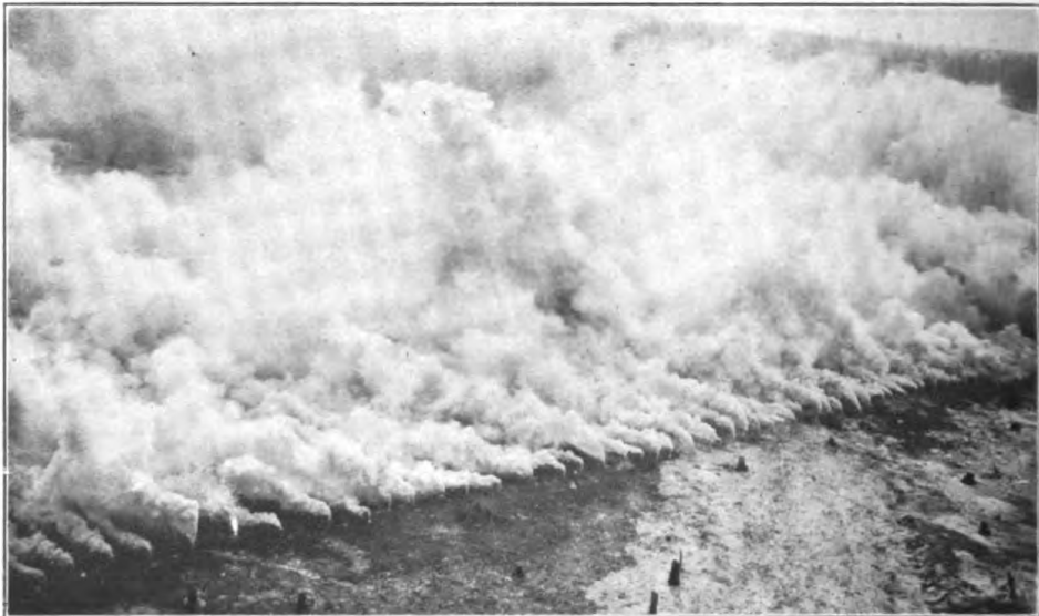
FIG. 3. THIS CLOUD, SET UP BY TOXIC CANDLES BURNING 650 POUNDS OF D. M., PRODUCED UNBEARABLE IRRITANT EFFECTS AND VOMITING IN OBSERVERS 3 MILES AWAY
