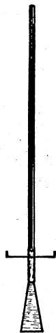
FIG. 15.—The spud, an effective tool for cutting off weeds with thick roots below the surface of the soil.
