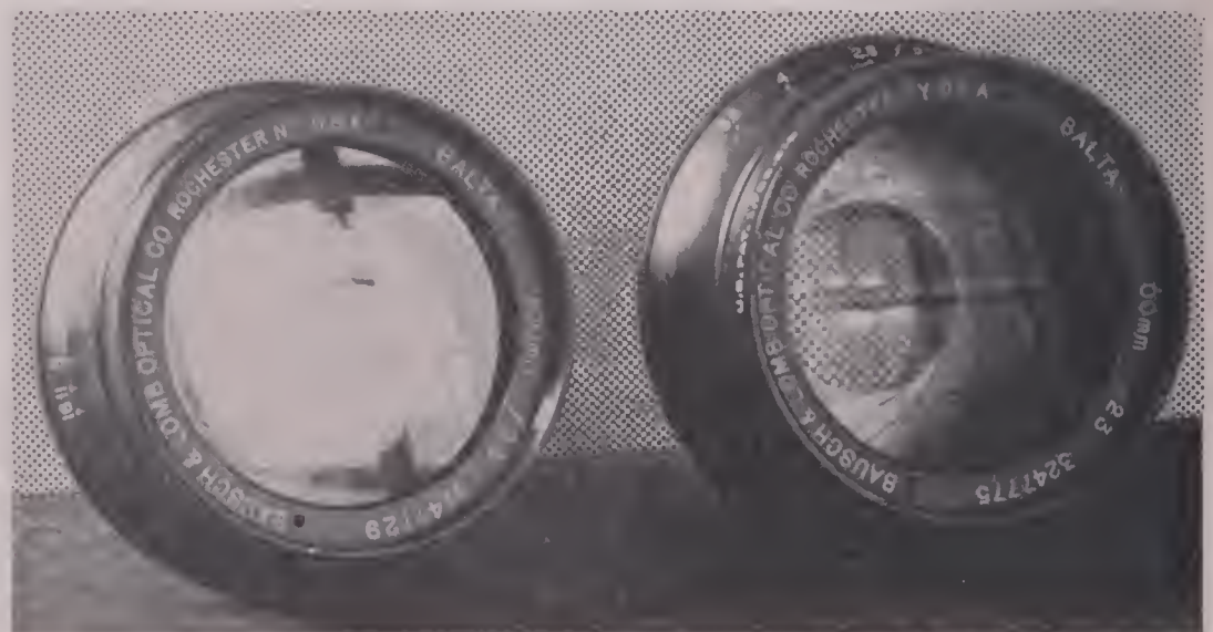
Fig. 5. An uncoated and a coated lens. The coated lens (right) clearly shows the diaphragm and the background.
