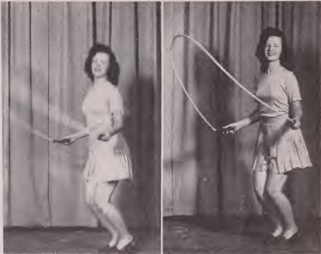
Figure 4 (left): Photograph taken from a strip of motion picture film, with illumination from photoflood lamps. Figure 5 (right): Single frame of motion picture film—taken with the subject illuminated by two flashtubes. Note that the motion is effectively stopped.
