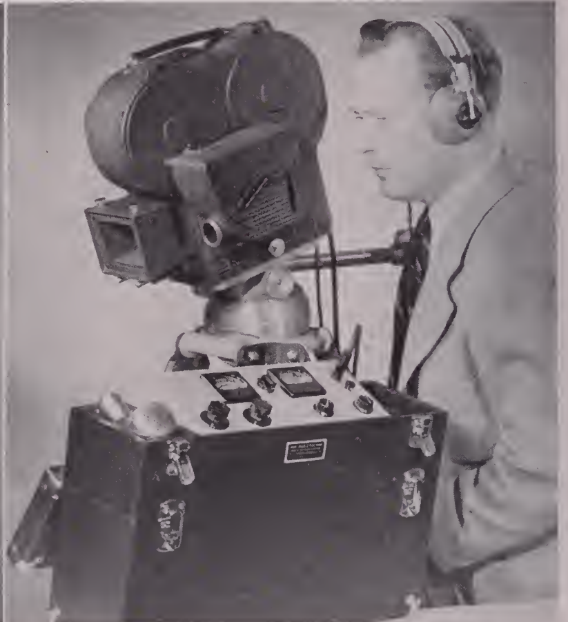
At left, a geared Veeder-Root footage counter indicates footage exposed, and can be re-set to zero. Right, the complete "Auricon-Pro" camera and equipment.
