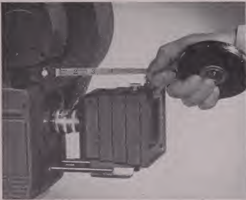
The new "Auricon-Pro" 16 mm. sound camera is designed for constant use and professional performance and results. At left, convenient stud above lens mount provides accurate measurement between camera and subject. At right, side cover is removed to show interior.
