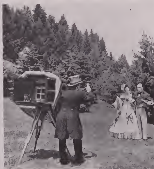
How a professional photographer of the 1870 period operated. His "portable" wet plate camera also contained a laboratory, where plates had to be developed immediately following exposure. This camera is one of the many in the Eastman collection.
