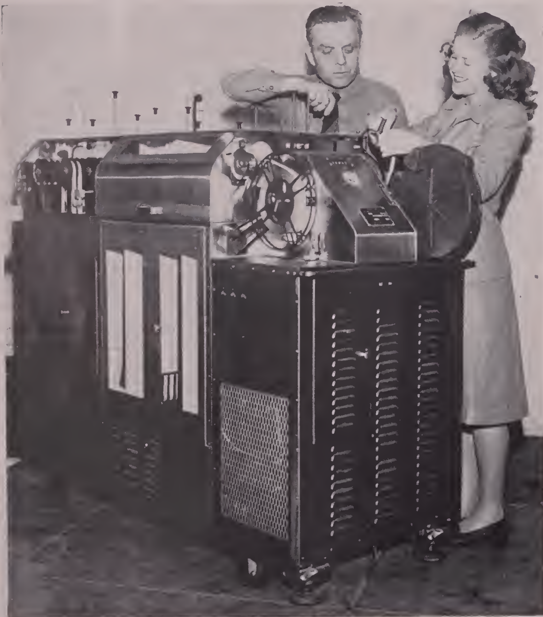
Houston portable film processing machine develops pictures of U.S.C. grid games within 10 minutes for showing to team at half time. Elbert Baldrige and Beverly Normanly are attaching film magazine.
