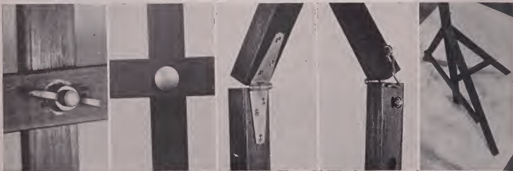
Details of assembly. Left to right: winged nuts enable the dismantling of the cross-beam without special tools; \frac{3}{8} in. carriage bolts, 2\frac{1}{2} inches in length, hold the cross-beam securely in place; hinges provide for portability of the unit, while . . . hooks and eyes hold the sections firmly in place; partial view of one stand, showing base construction.
