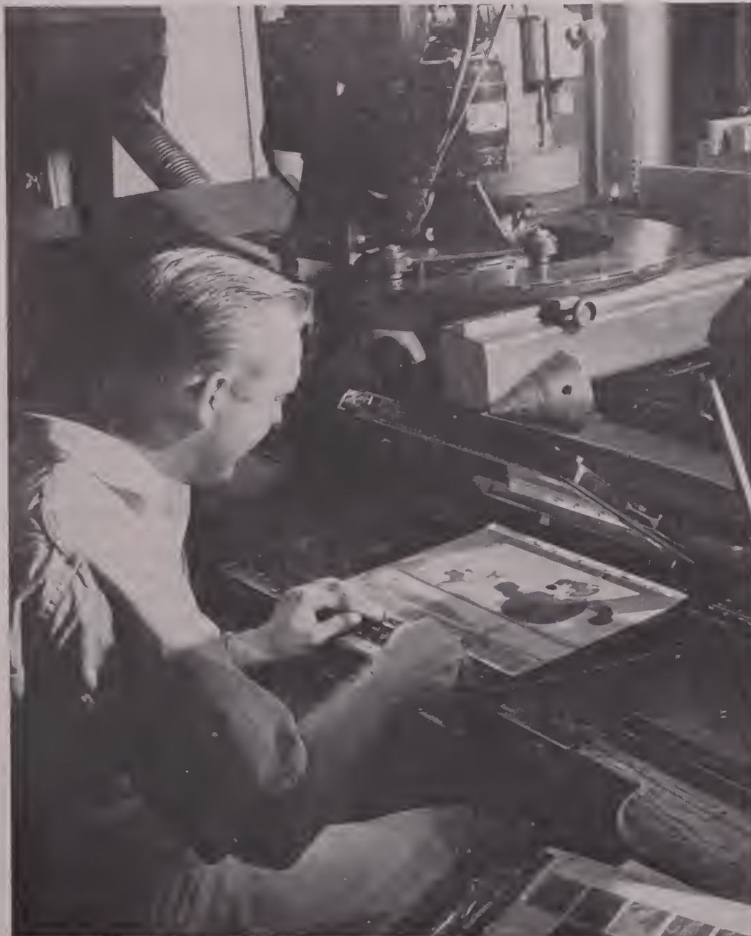
The photographing of a cartoon feature is a lengthy process, since each individual celluloid painting has to be photographed separately on top of its corresponding background. The operator must clean each cell carefully with an air hose before exposing it.
