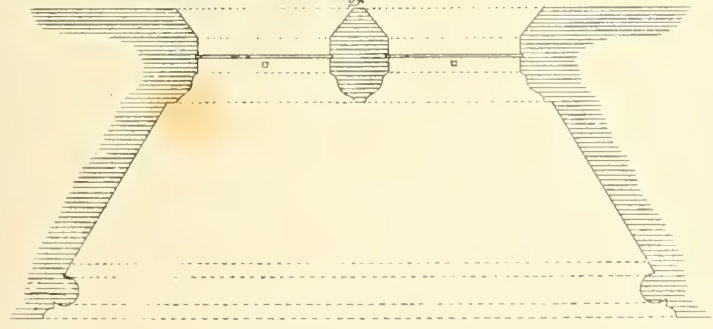
Window S. Aisle of Waltham Abbey Church, Essex.
