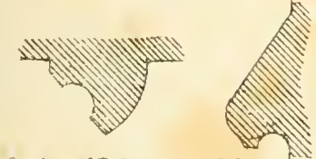
Section of Dripstone and String 1/2 nd Scale
