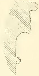
Section of lower cap.
