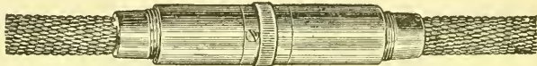
FIG. 3. One-quarter-inch hose with improved couplings. From Forbush, report Massachusetts Board of Agriculture, 1898.
