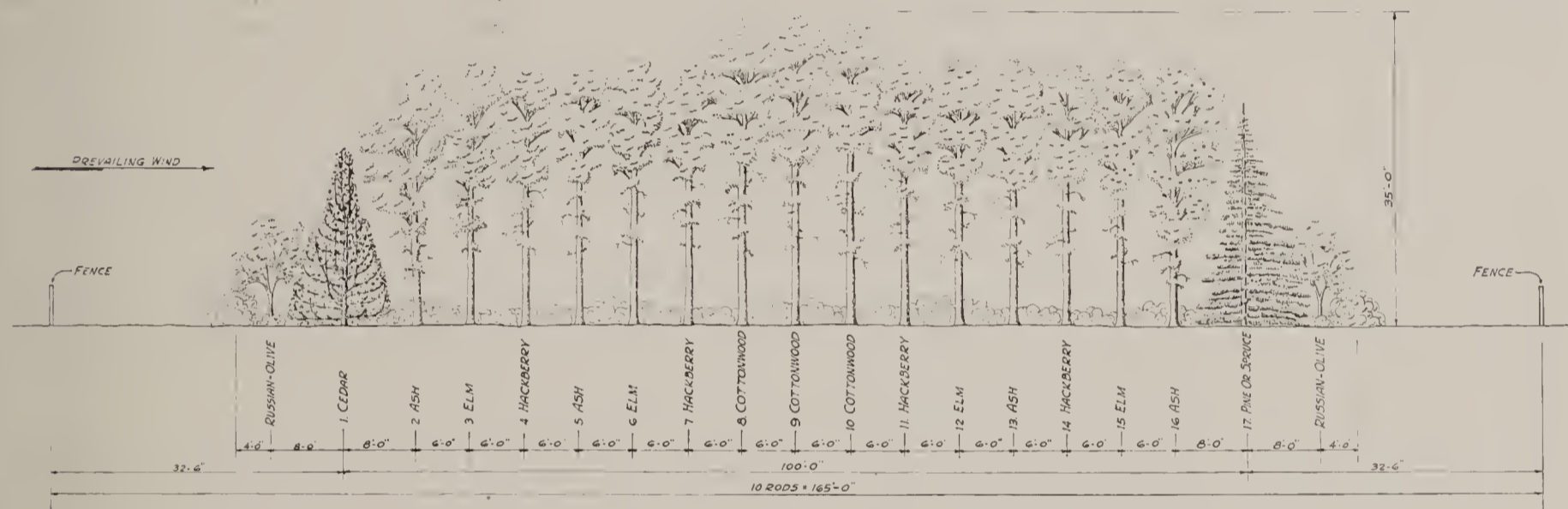
FIGURE 5.—Cross section of 17-row shelterbelt on 8-rod strip, with sand trap and roadway on either side.
