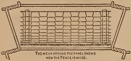
THE MESH AROUND THE PANEL SHOWS HOW THE FENCE IS MADE.
