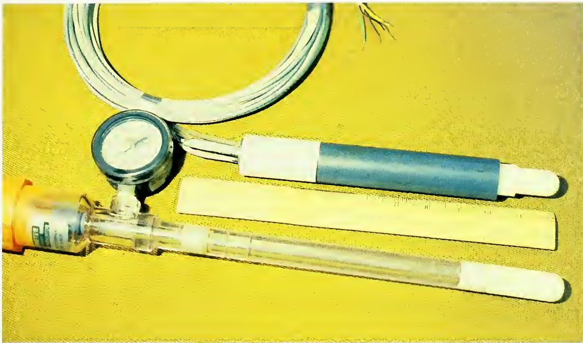
Figure 31. A transiometer (top) prior to installation adjacent to a tensiometer.
