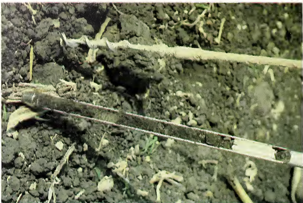
Figure 29. Probe used for soil sampling.
