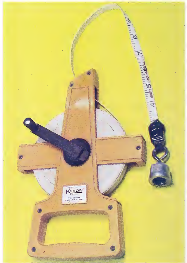
Figure 7. Fiberglass tape with a popper.
