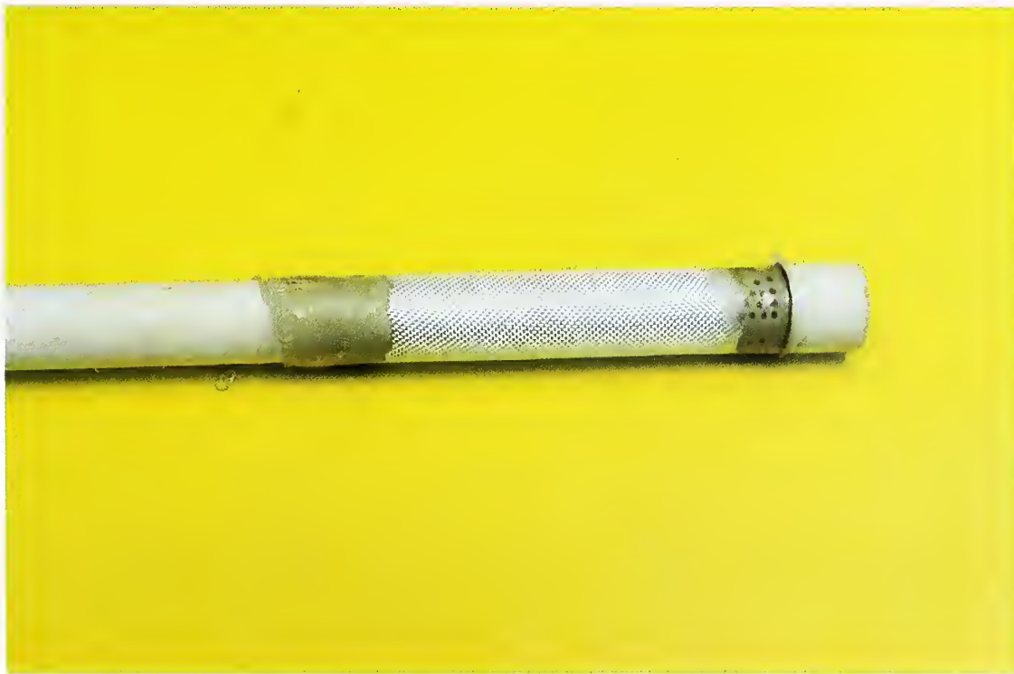
Figure 12. An in-lake well with a fiberglass screen.
