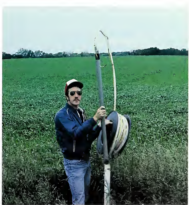
Figure 6. Bladder pump with trifluoroethylene tubing.
