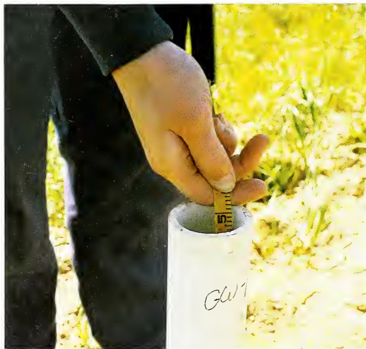
Figure 19. Measuring water levels.
