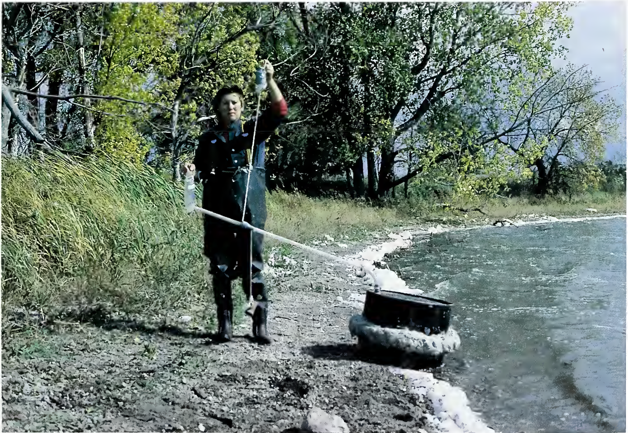
Figure 13. A seepage meter ready for installation.
