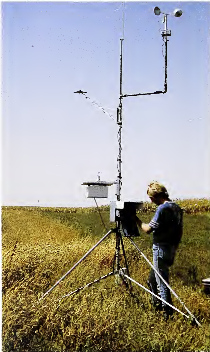
Figure 25. Portable automated weather station.
