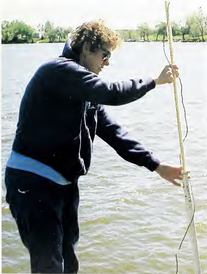
Figure 18. Measuring water levels with a beeper pole.
