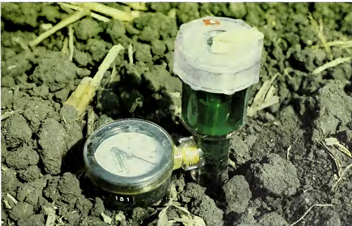
Figure 28. Tensiometer installed at a farmed field site.
