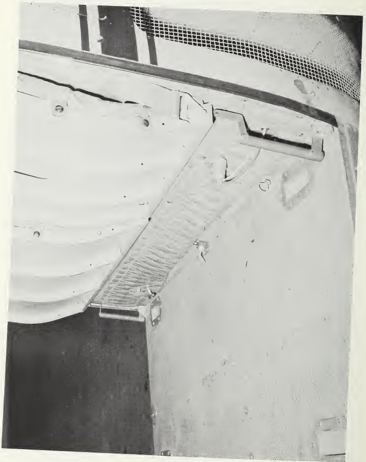
REAR SAFETY HANDRAIL FOR HELITACK CREW MEMBERS AND SAFETY HARNESS ANCHOR IN CENTER OF SEAT - BELL RANGER MODEL J
