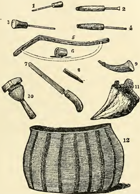
Tools of an oriental carpenter. 1, 3, 4. Drills. 2. Chisel. 5. Handle of a drill. 6. Nut held in the hand while the drill revolves. 7. Saw. 8. Punch. 9. Horn of oil. 10. Mallet. 11. Bag for nails. 12. Basket to hold tools.
