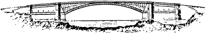
TELFORD'S PROPOSED CAST IRON BRIDGE.
