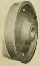
BACK OF FINISHED CENTER, READY FOR TIRE
