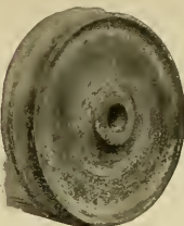
FRONT OF FORGED CENTER, BEFORE SURPLUS METAL WAS SHEARED OFF.
