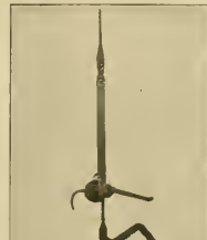
DEVICE FOR HOLDING DRAWBAR WHILE YOKES ARE BEING RIVETED ON
