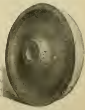
BACK OF FORGED CENTER, AFTER SURPLUS METAL WAS SHEARED OFF.
