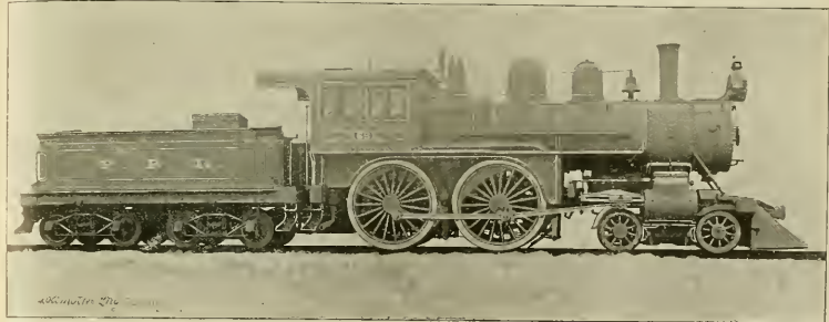
NEW CLASS "P" EXPRESS LOCOMOTIVE, WITH 8- 1 / 2 -INCH DRIVERS, FOR PENNSYLVANIA R. R.
