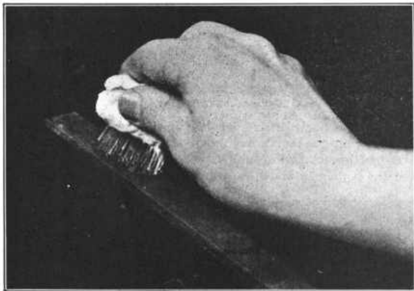
FIG. 8.—The hot-iron test. The curd is ready for pressing when it sticks to a hot iron and is drawn out in threads which break when about \frac{3}{4} inch long.
