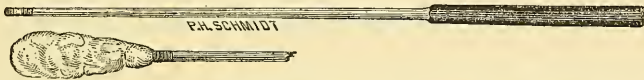
FIG. 116.—Straight whalebone stick, with notched end, for wrapping cotton around end, as shown in smaller cut.
