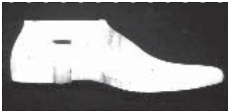
Fig. 4-35. SACH foot. A: keel, B: cushioned heel, and C: belting to prevent end of keel piercing through foam at the toebreak.
