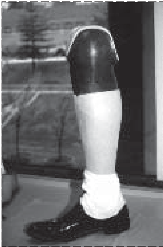
Fig. 4-28. Supracondylar thermoplastic patellar tendon bearing, total contact socket (PTB-TCS). The medial and lateral walls extend above the condyles and indent to provide suspension, mediolateral stability, and rotational control.
