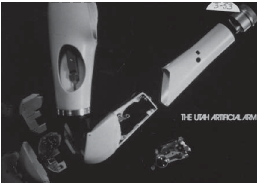
Fig. 3-53. The Utah myoelectric prosthesis. Photograph: Courtesy of Motion Control, Inc., a division of IOMED, Salt Lake City, Utah.
