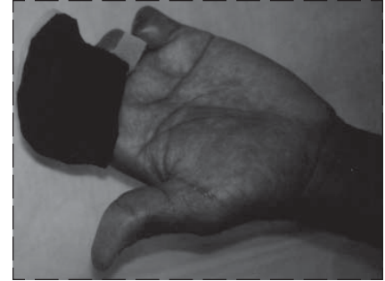
Fig. 3-11. Palmar surface of the prosthesis shown in Figure 3-10. This prehensile surface is coated with foam rubber, which increases grasping friction.
