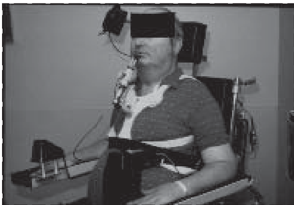
Fig. 5-8. Chin control. This individual with C-4 quadriplegia uses chin control to steer and to recline his power wheelchair and to operate an environmental control unit (ECU) with an infrared interface to a speaker phone, television and light controls.
