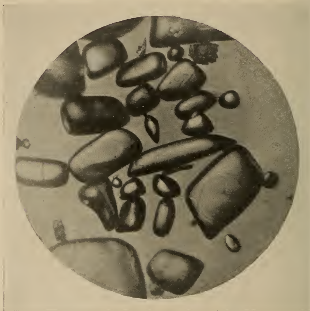
FIG. 1. Grains of crushed Iceland spar rounded by solution in warm hydrochloric acid. Note that the smallest grains are the most nearly round. Transmitted light. Magnified 70 diameters.
