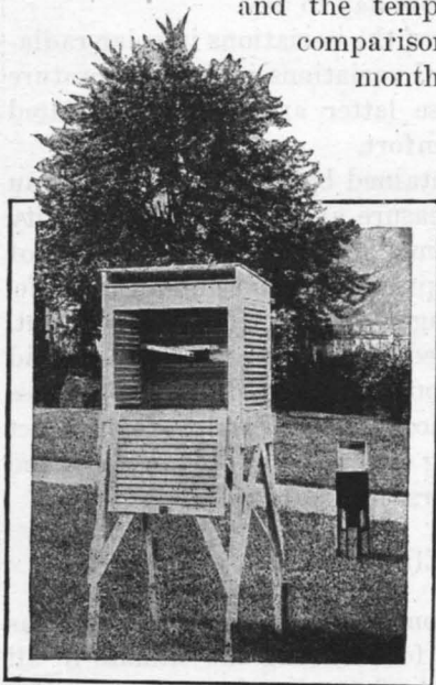
FIG. 7.—A cooperative weather observer's equipment: Maximum and minimum thermometers in a lattice-work shelter, and a standard 8-inch rain gauge.
