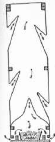
FIG. 4.—Cross section of a large fly trap for use in windows.
