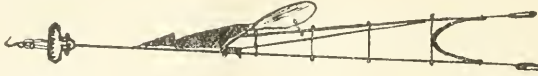
Plan of plough showing curved over end of breast and angle it forms with beam.
