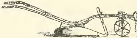
Plough suitable for light land, having a long breast much curved over at end and lying close to bottom of furrow.
