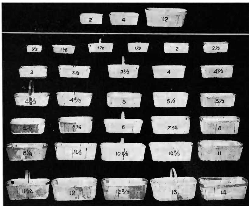
FIG. 5.—Above: Two, four, and twelve-quart Climax or grape baskets. Shipments of other sizes in Interstate trade are prohibited by law. Below: Thirty-one types of Climax baskets in general use in 1917, before the establishment of standards
