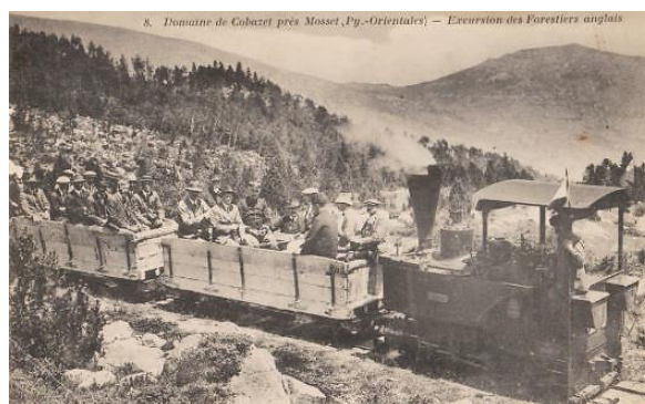
Decauville 0-4-0, Type 1, 3,250 tonnes empty, No 412 of 1904, 'Steatite'
