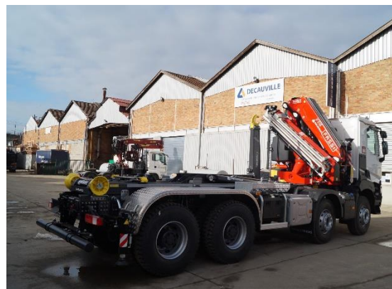
Marrel roll-off skip truck with a Fassi crane at the Decauville factory in Corbeil-Essonnes, 2023 (photo NearEMPTiness , CC BY-SA 4.0 )
