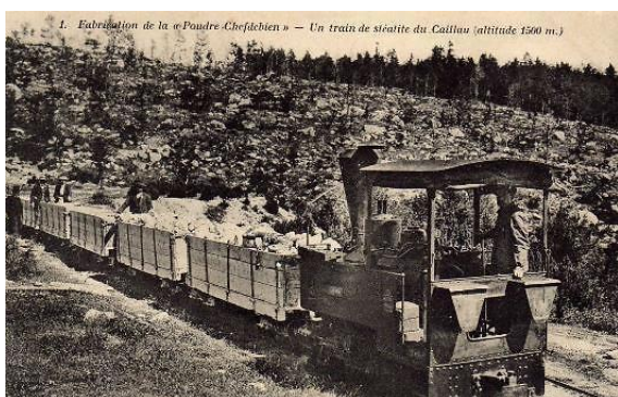
Decauville 0-4-0, Type 1, 3,250 tonnes empty, No 412 of 1904, 'Steatite'
