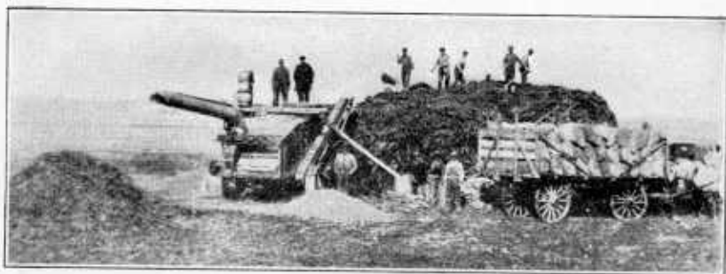
FIG. 12.—Rear view of an ordinary separator fitted to thrash beet seed. A crew of 10 men can thrash 30,000 pounds of seed a day, and two men can haul the thrashed seed to the warehouse.
