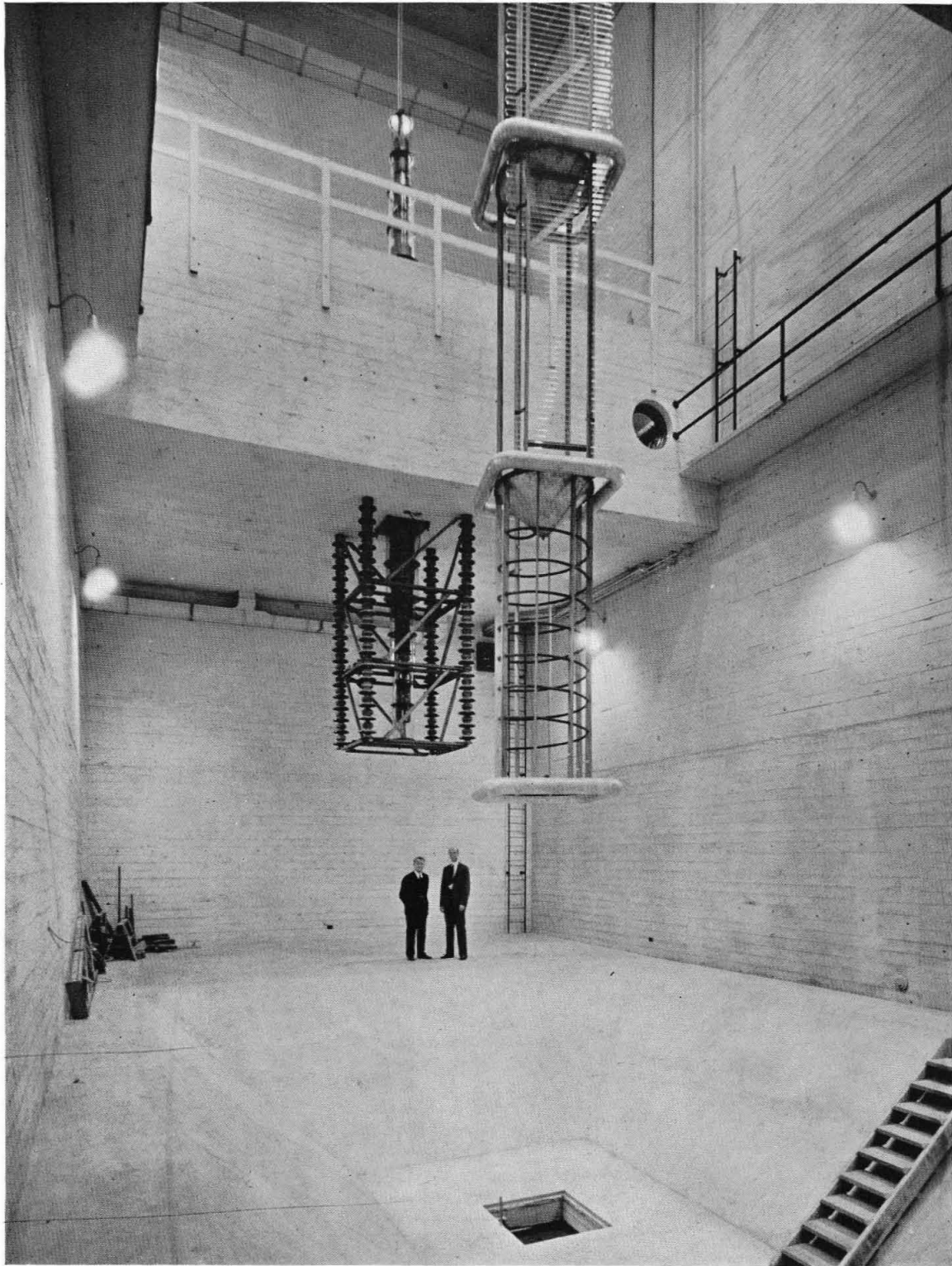
DR. LAURITSEN AND DR. MUDD STANDING BENEATH THE NEW MILLION VOLT X-RAY TUBE
