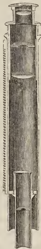
Draw-tube fitted with Erector.
