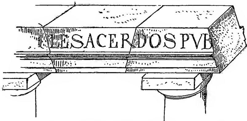
212—Architrave and frieze in one piece, built as a flat arch, at Pompeii. (From Hdbch.—Etr. und Röm.)
