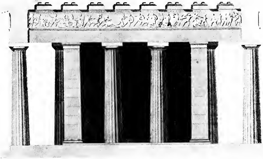
127—Cross section of the Theseion, showing "Ionic" frieze. (From S. and R.)
