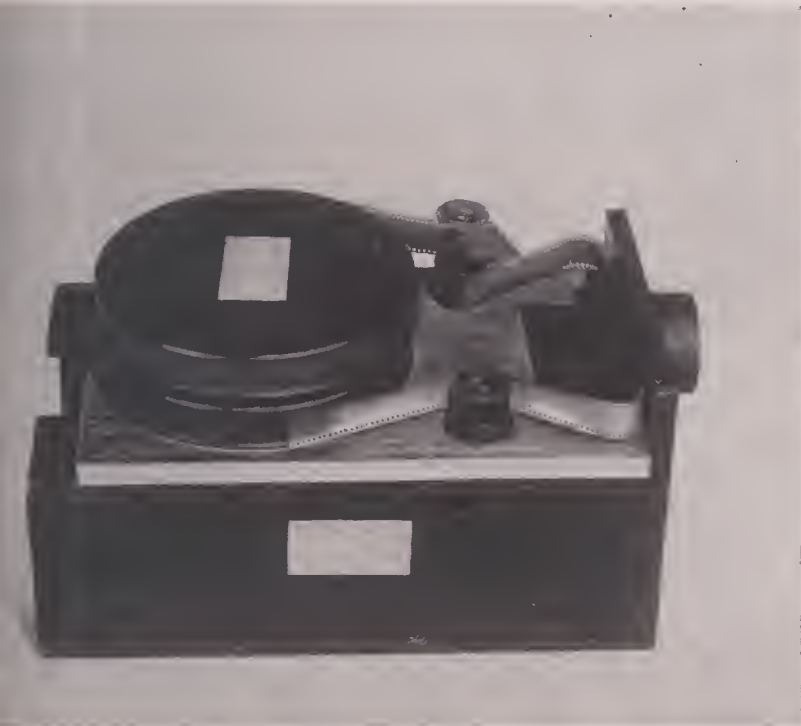
4—Cartridge-loader model. This design suggests use of interior magazines for either 1000-ft. or 2000-ft. rolls of film, utilizing a removable compartment to include two stacked magazines in horizontal position. (Housing not shown.) Included is rack-back and finder prism housing mounted to slide vertically behind lens.
