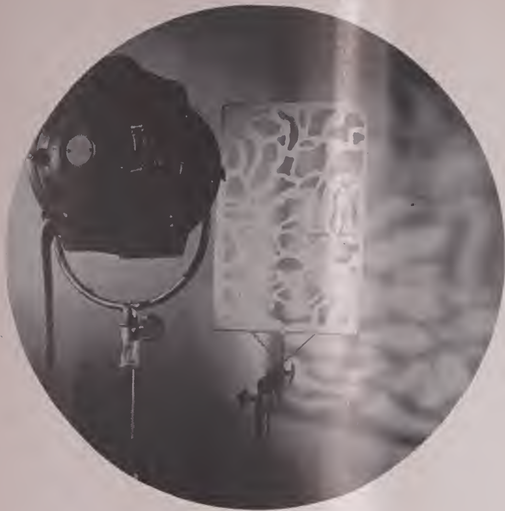
THE CUKOLORIS, when interposed between a lighting unit and a wall breaks the light up into interesting patterns of light and shadow. Here both lamp and "cookie" are placed much closer to wall than in normal use, in order to more graphically demonstrate the effect obtained.
