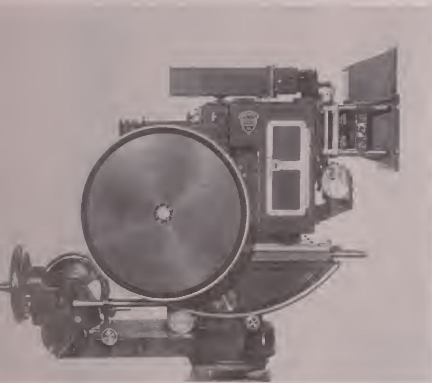
FIG. 1—Exterior side view of the new VistaVision camera, showing 2000 ft. vertical film magazine (with cover removed). After exposure, film is taken up in separate magazine on the other side of the camera. Note tilt mechanism as integral part of the camera base unit. Camera was built by Mitchell, gearhead by Paramount.
