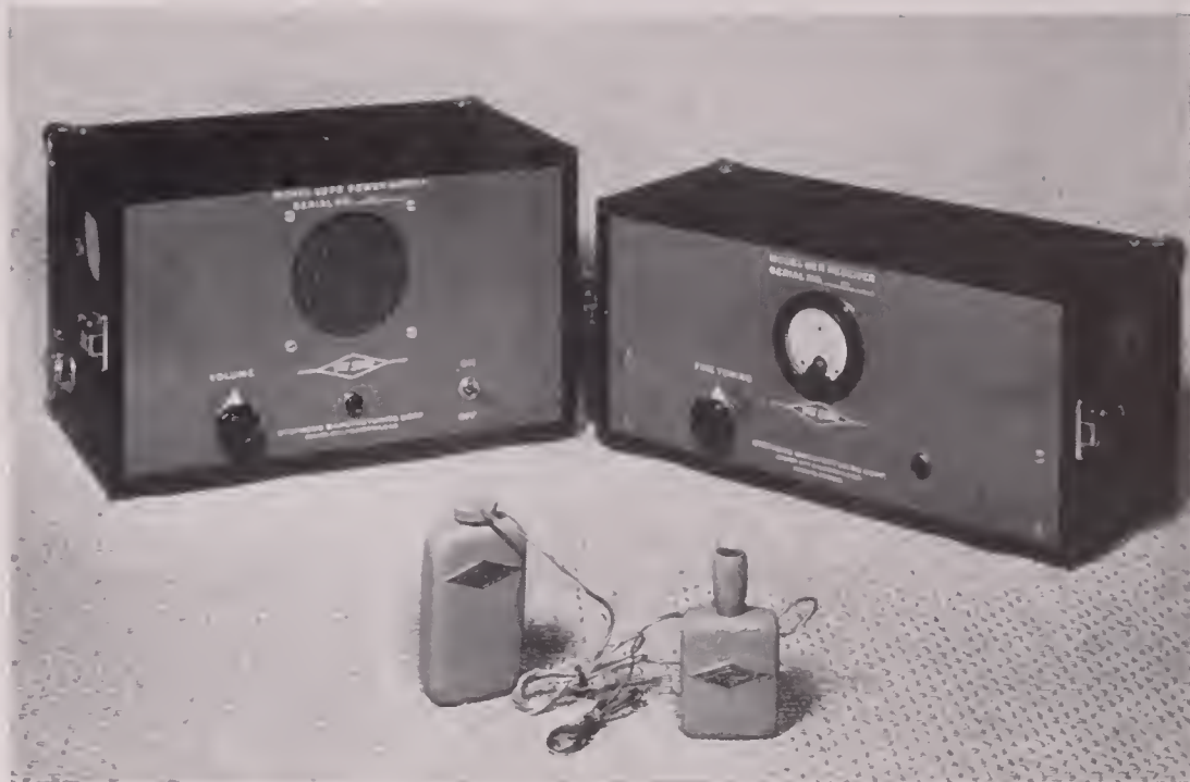
STUDIOS are using this wireless microphone equipment for sound stage communication between technicians, also to eliminate the mike boom in certain types of shots. System includes power supply and monitor speaker in one unit, receiver, combination mike and transmitter, and small battery to power transmitter. Also included but not shown here is a vertical receiving antenna mounted on floor stand.
