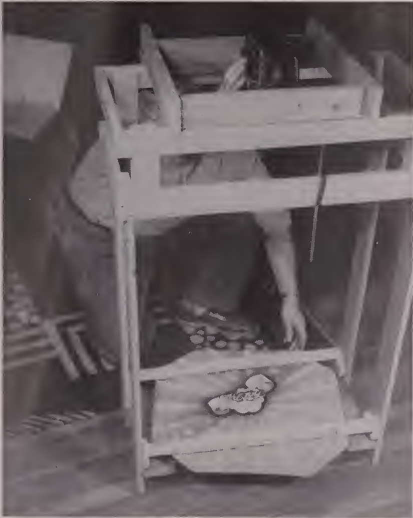
FIG. 1—HOMEMADE TITLER constructed by author was used in photographing the 8mm film leaders which were awarded the winners in the New York City 8mm Club's 1953 film competition. Text on clear celluloid panels was photographed superimposed over decorative revolving background.
