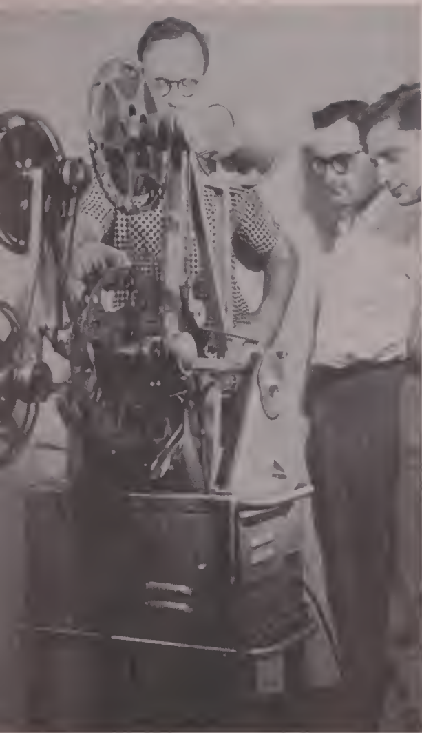
THE ROUGH cut of a TV film is reviewed in the Moviola by the editing staff.
