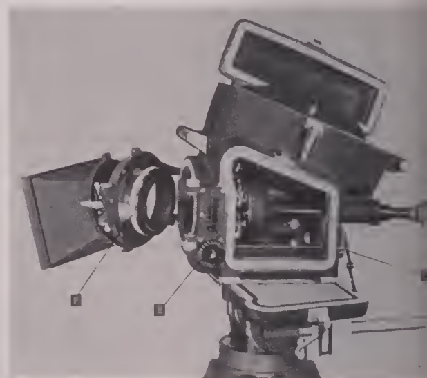
3 EXTERNAL focusing knobs (D and E) afford follow focus control of blimp-mounted Arriflex, while a unique focusing scale (F) affords quick check of f/ stop through small window just above focus control knob (E).
