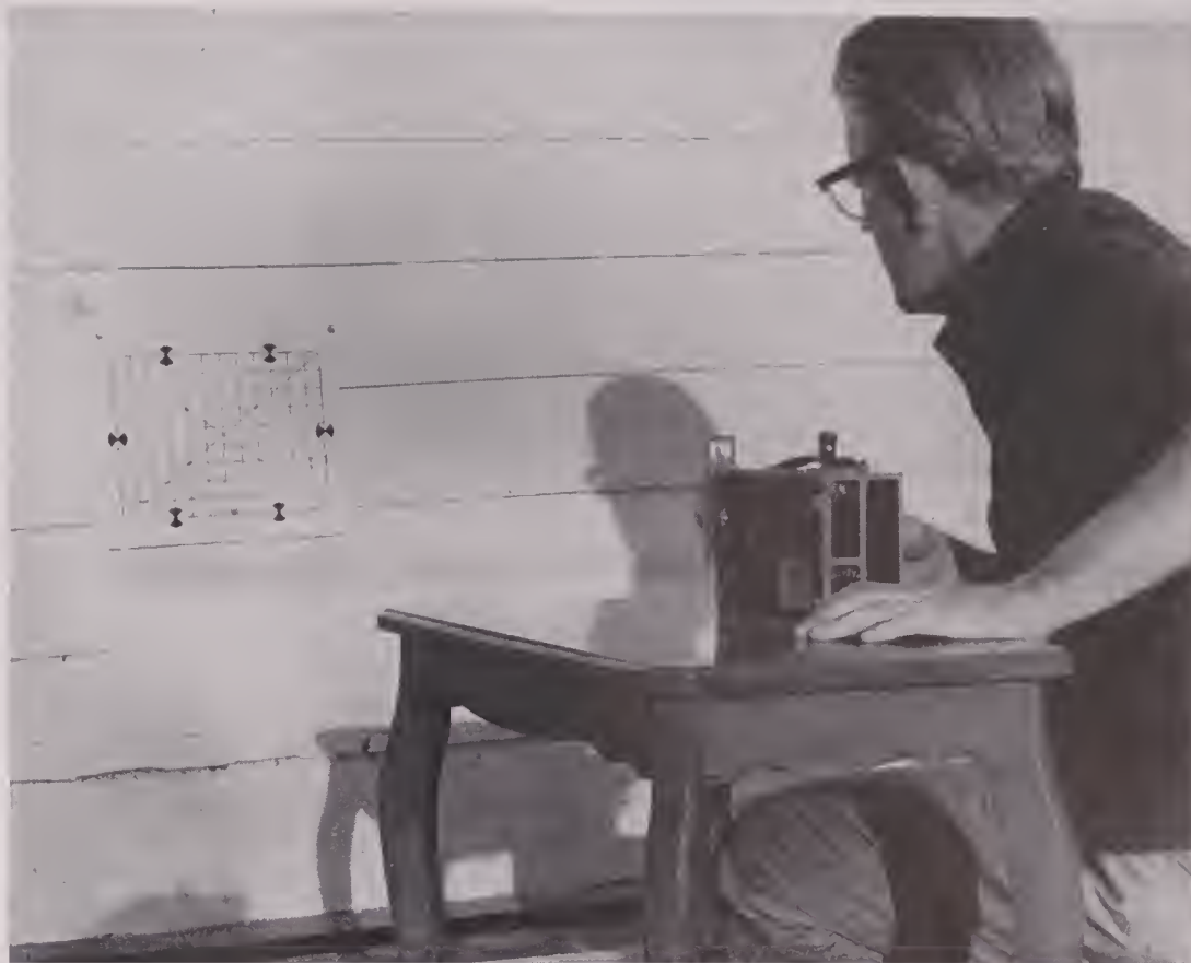
STEADINESS of intermittent movement and viewfinder accuracy may be checked at the same time, by photographing a chart such as shown here. The procedure is described by author in the text.
