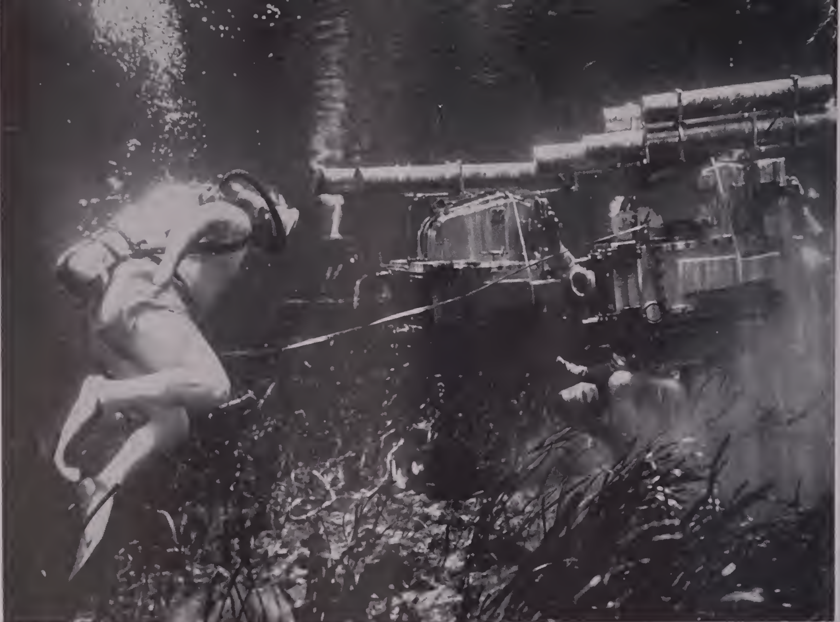
RUNNING A TAPE before starting to shoot a scene for MGM's "Jupiter's Darling" at Silver Springs, Florida. The two underwater blimps house Mitchell cameras with 1,000-foot magazines. One camera shoots CinemaScope, the other wide-screen. Camera oper-
