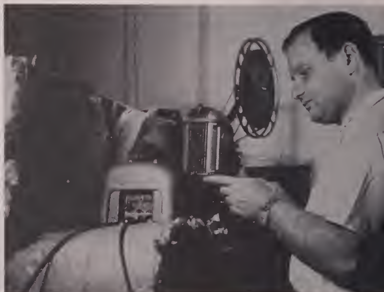
PROJECTING a rough cut work print from a soundproof booth while recording sound effects in sync with the picture.
