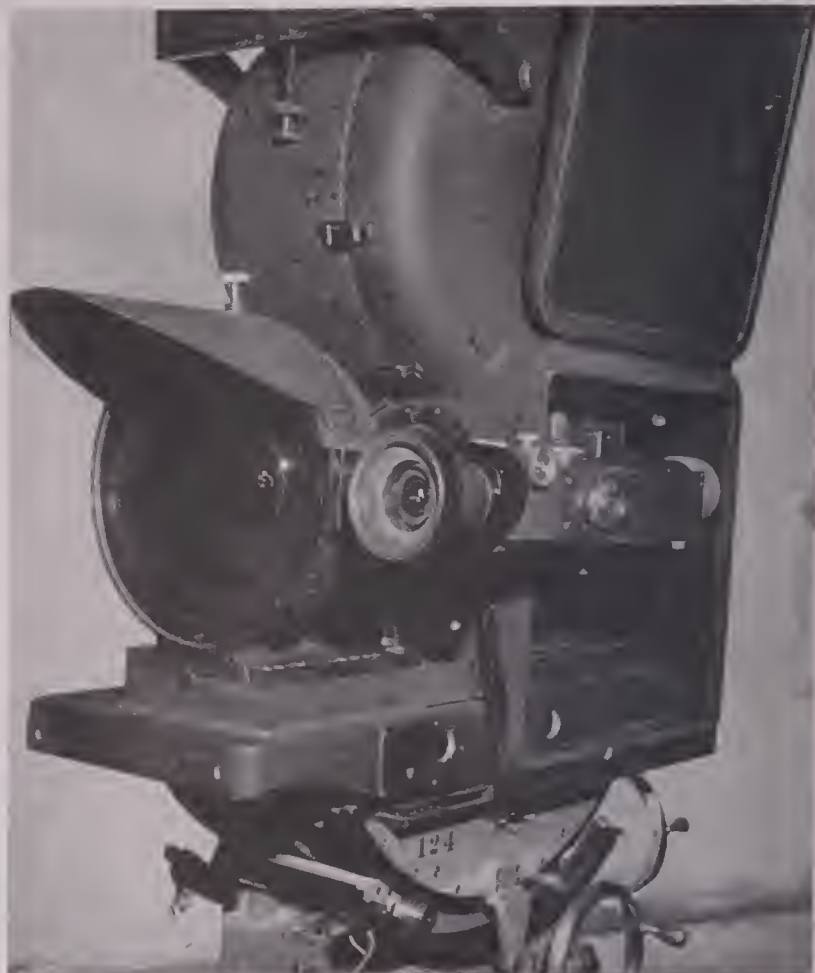
TODD-AO camera, showing the 128 degree “bugeye” lens and the companion wide-angle viewfinder. Camera is not much larger than a Mitchell and is about the same weight, due to use of new type fiberglass insulation in blimp. Camera uses 65mm negative.
