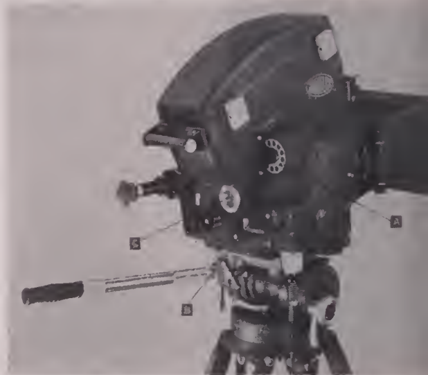
2 AT REAR is telephone-dial type threading knob (A), and windows affording observation of tachometer (C) and footage counter (B).
