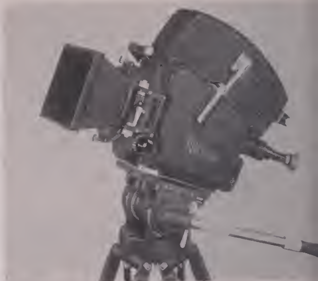
1 OUTSTANDING feature of the New Arriflex is the new Arri blimp, designed especially for the camera using 400 foot magazines and sync motor.
