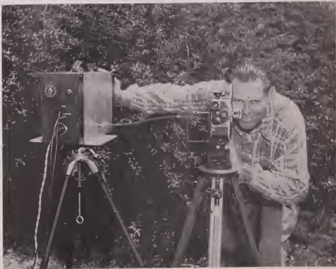
FIG. 4—An early model of author's magnetic film recorder is shown here coupled to a 16mm Bolex camera by means of flexible cable and a reversing gear. Camera operator is Earl Everley of Long Beach (Calif.) Camera Club.
