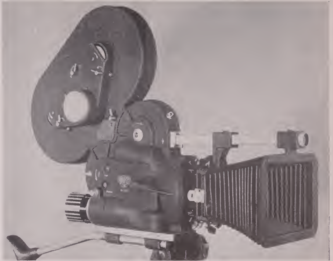
4 FOR 16MM PHOTOGRAPHY, Arriflex offers its latest model 16mm camera featuring such improvements as "button-on" 400 ft. external film magazine, divergent 3-lens rotary turret, registration pin, and built-in electric motor drive.
