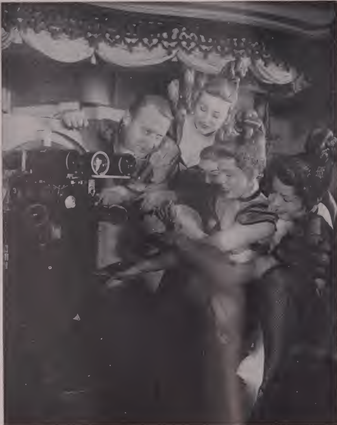
THE TRI-LENSED Cinerama camera is explained to a bevy of French can-can girls at the famed Lido in Paris by author Joseph Brun, who photographed the girls for "Cinerama Holiday." View of camera is from rear, shows the finder tubes—one for each of the three camera lenses.
