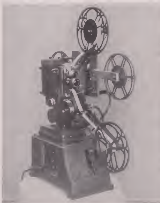
FIG. 4—Another Ampro sound projector adaptation. Playback unit is mounted at rear, and sound plays back through the projector augmented with a pre-amplifier.
