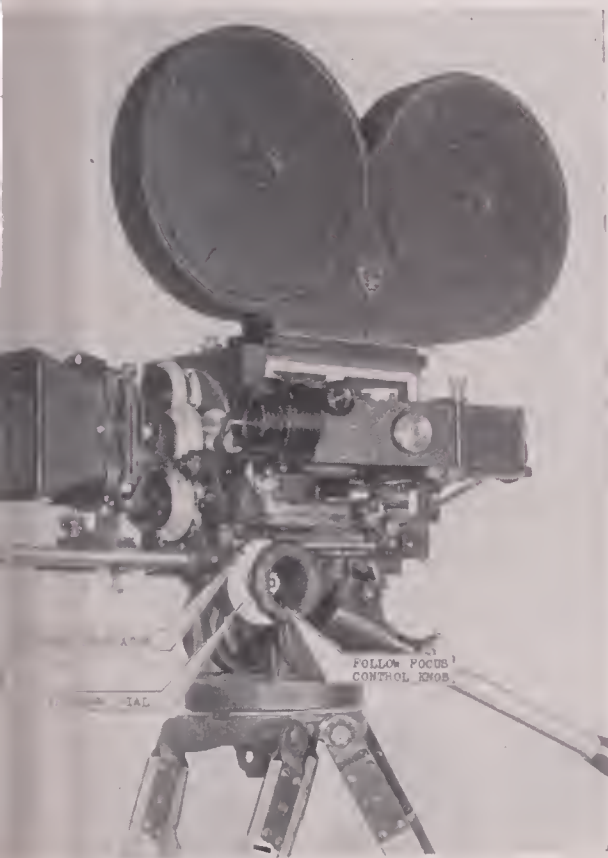
FIG. 1 —Follow-focus attachment installed on Mitchell NC 35mm camera, which enables it to be used for moving shots at various distances, and gives the cameraman full control of both picture framing and lens focusing through operation of a single follow-focus control knob.
