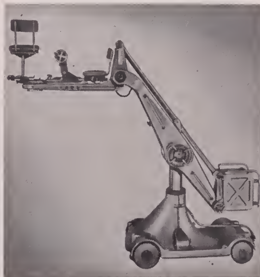
MODEL BT-1 CRANE has power drive, hydraulic lift. Provides lens height from 2' to 10'. Developed for Motion Picture Research Council.
