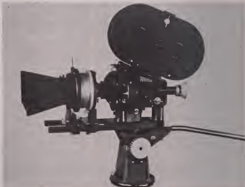
FIG. 3—Adaptation of CinemaScope lens to present 3-lens Arriflex 35mm cameras. C-lens is mounted on special cradle which slides before camera lens on rails.
