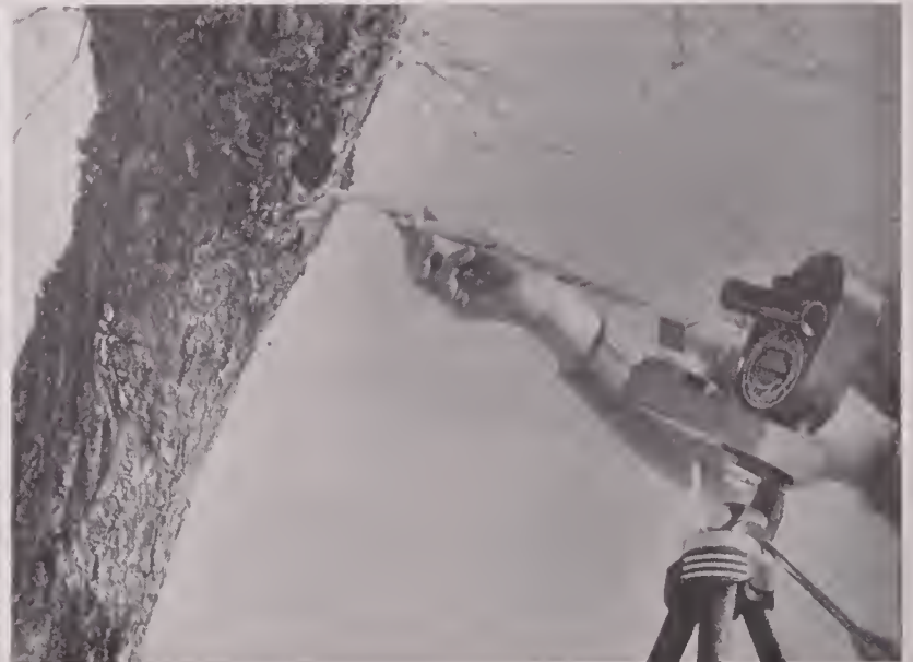
FIG. 4—The remote controlled camera must be pre-focused and framed so the desired bird action takes place where camera will record it. Here a ruler is used to determine correct focusing distance.
