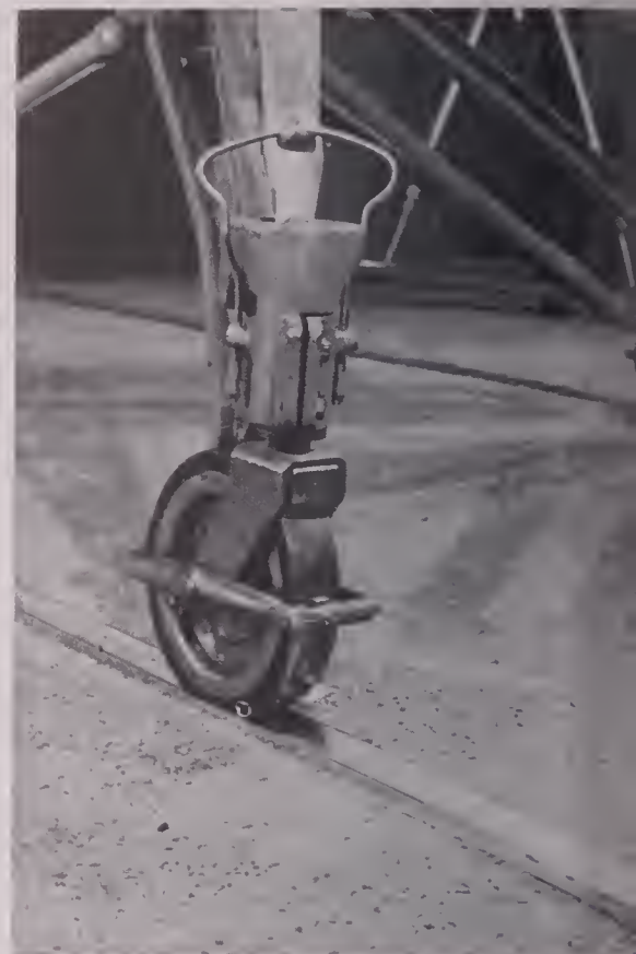
TRACKS for the dolly wheels make for smoother dolly travel. Here a commercial-type dolly designed for both amateur and professional cameras, riding a channel track made of light-weight metal that is generally available in heavy hardware stores.
