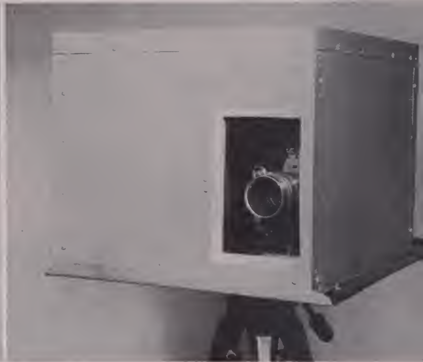
FIG. 2—The same unit shown at left covered with a blimp made of Celotex. Equipment and blimp rest on metal base which has fitting for mounting on conventional camera tripod.
