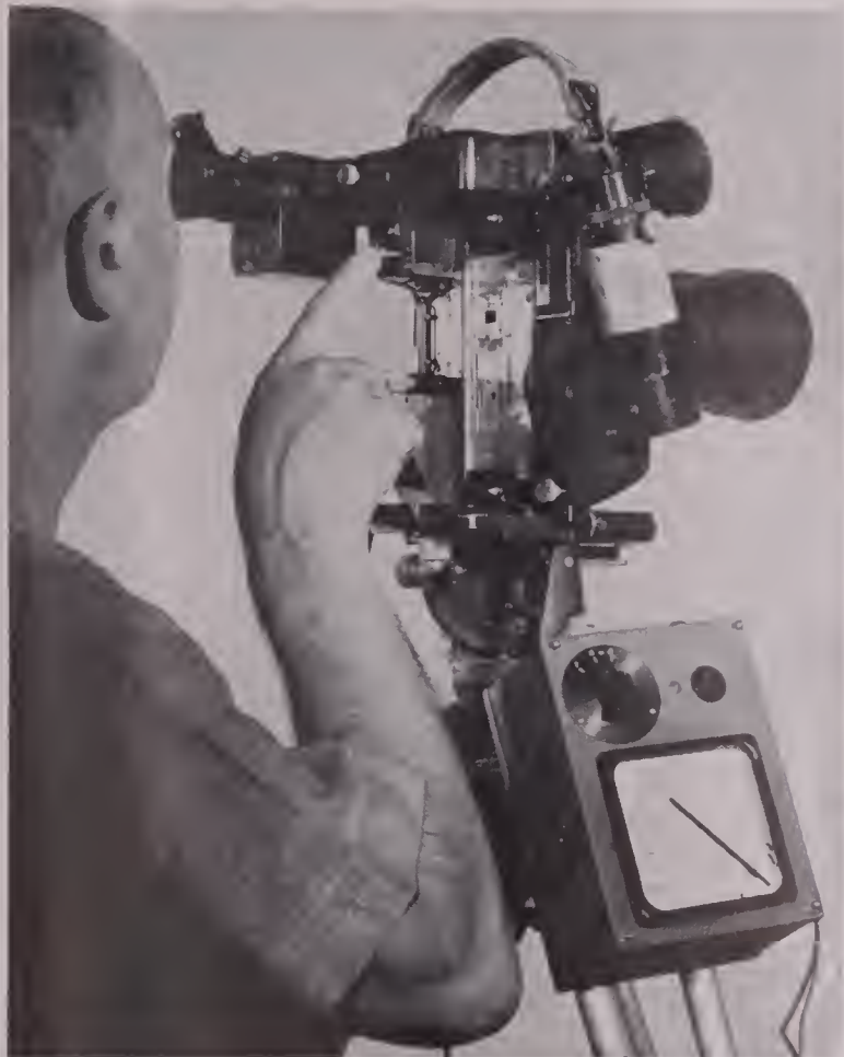
WHEN MOUNTED in the Eclair Camerette, the Sensitoflex is known as the Came-Radar. Here operator is shown moving the finger-tip control that moves the tiny photocell over the groundglass within the finder—an operation the cameraman observes through the finder eyepiece. Attached to tripod (lower right) is the photometer which records the light response of the Came-Radar.
