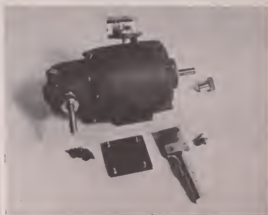
THE unmounted motor, showing (in foreground) the additional parts that had to be added to permit mounting on the B&H "70" camera.
