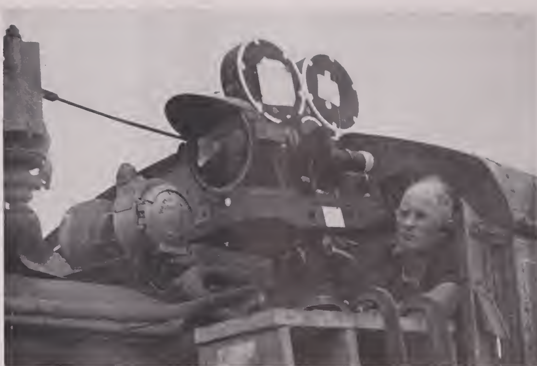
ONE OF THE unique camera mountings employed by Floyd Crosby, ASC, who directed photography of the second unit of the initial Todd-AO production, "Oklahoma." Here "bugeye" lens was used on camera to make a running shot from a moving locomotive on a rail line near Nogales, Arizona.
