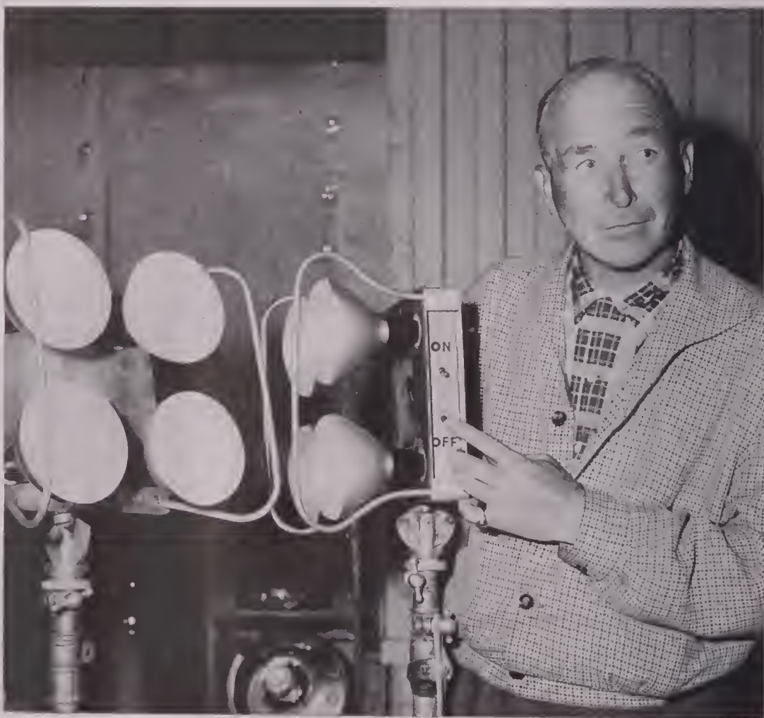
AL LANE, set electrician at MGM studios in Hollywood, points out rugged quad-lite which that studio engineered and built for standard set lighting use. Quads have sockets for four photoflood lamps, switches to control lamps in pairs. Housing is all aluminum and has regulation tilting and swivel fitting for use on regular lamp standards. Heavy wire brackets at either side of lamps protect them from damage.
