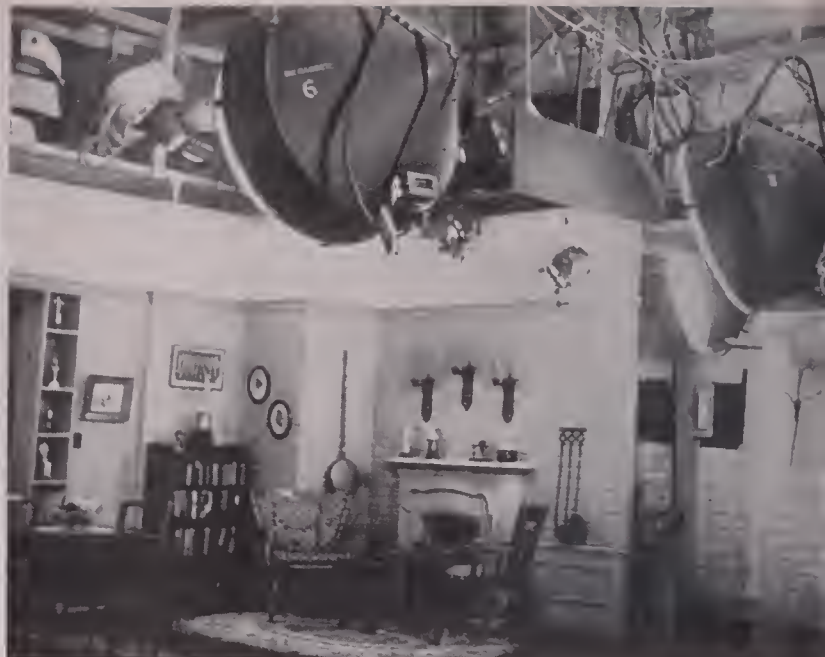
HERE IS the familiar living room set of the Mortons, next-door neighbors of George and Gracie. Prominent are the two cone lights suspended from ceiling which supply the main fill light. Other units augment the illumination of the cone lights.
