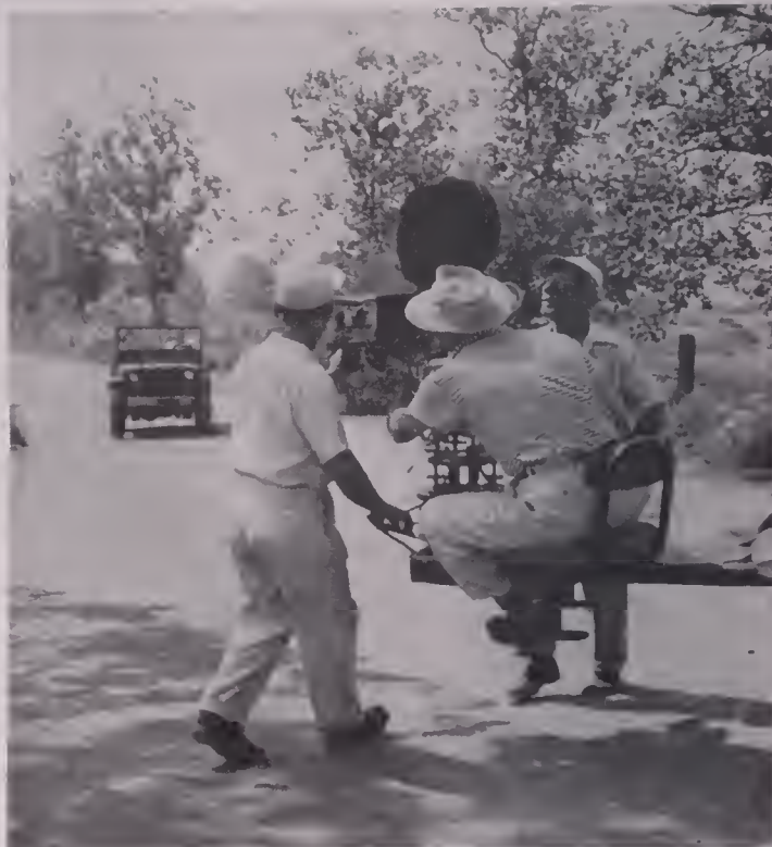
WITH CINEMASCOPE camera on boom, Sam Leavitt's camera crew shoots a scene on location. As Jeep approaches camera, assistants on either side of camera move the boom, enabling operator to follow the action.
