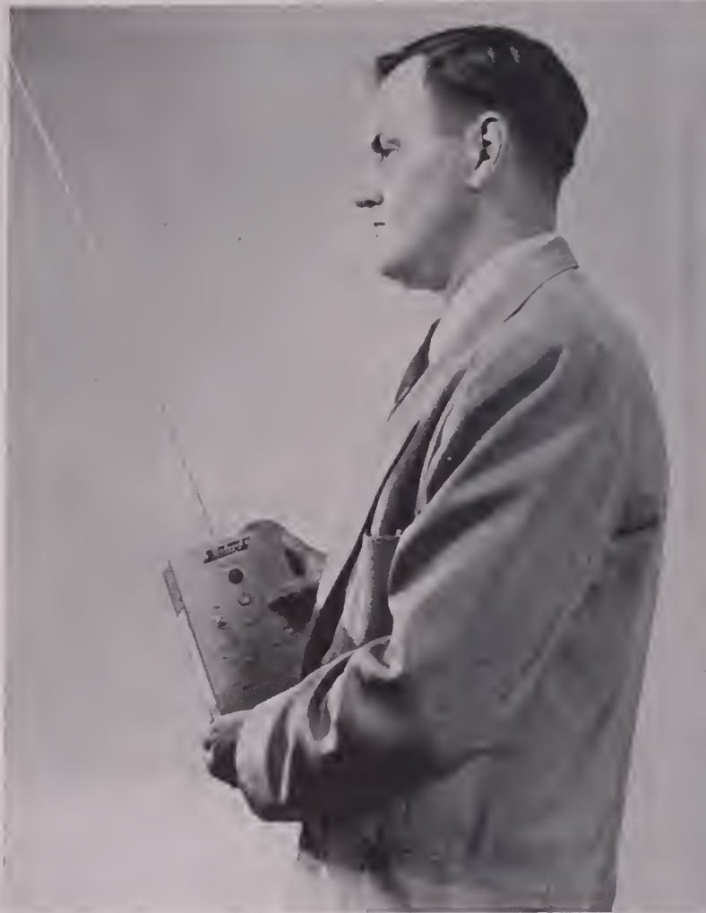
REMOTE CONTROL transmitter in hands of author. Pushing a button creates radio impulse which is picked up by receiver connected to camera control unit. Transmission range is 1 mile.
