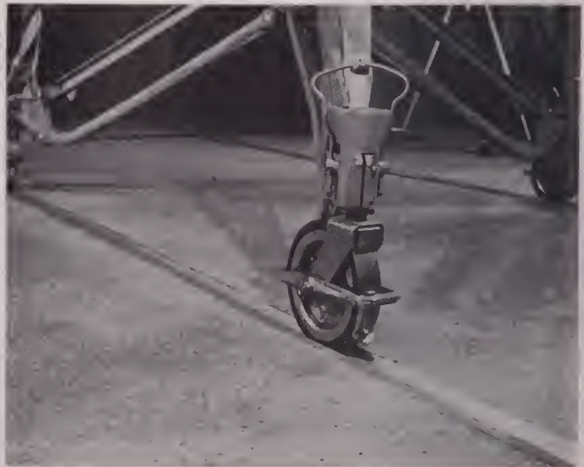
CHANNEL of tracks should accommodate dolly wheels without binding, be deep enough to hold wheels during camera shots.
