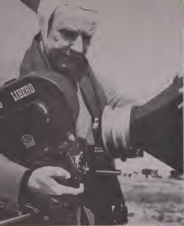
FIG. 1—CinemaScope lens swings readily out of way to permit setting stop and focus of camera lens. Pictured is the first Arriflex Cinema-Scope camera adapted for Astra Pictures, Italy, used by cameraman Mario Gaveri in making helicopter shots for "Lost Continent" in Indonesia.
