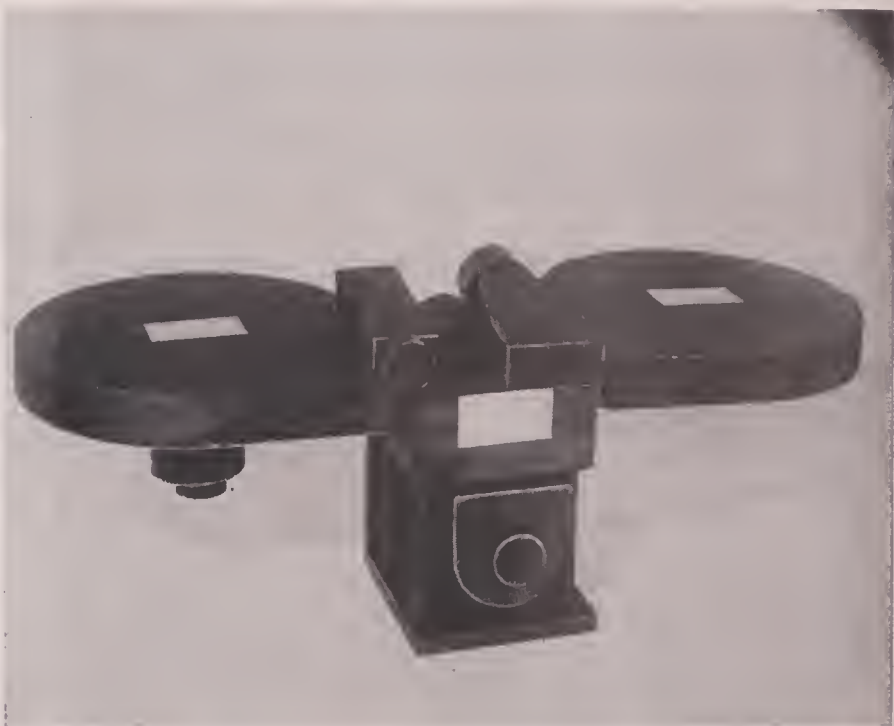
FIG. 5—Butterfly type. Where shooting requires minimum height of camera, this design finds immediate acceptance. Separate 2000-ft. magazines mount horizontally on either side of camera. Finder and viewing tube are located on top, center. Camera racks up and down for lineup through taking lens. Viewing tube can be shifted also.
