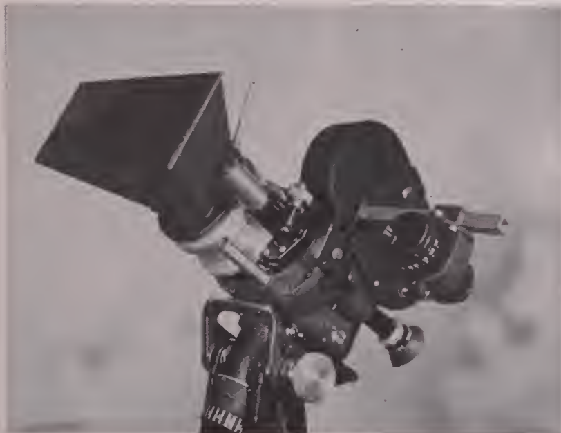
FIG. 2—In this adaptation, regular 3-lens turret is replaced by single-lens turret plate which also provides swing-mount for the CinemaScope lens. Note special finder on bracket.
