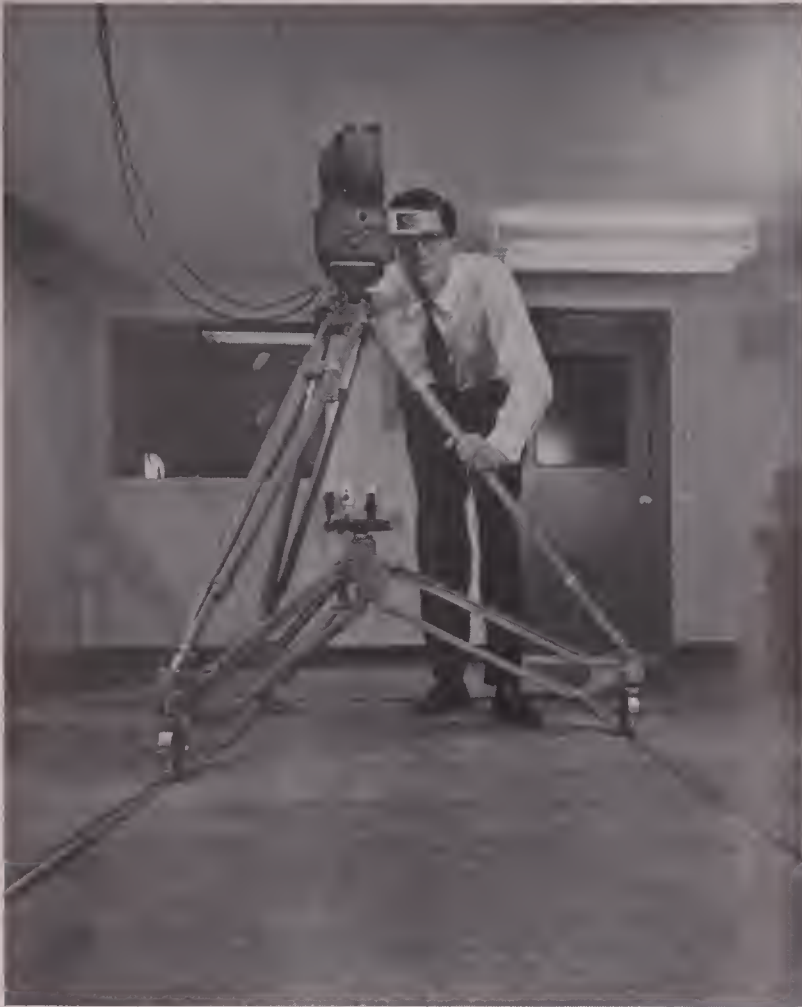
LENGTHS OF lightweight channeled iron or aluminum laid on floor provide effective tracks for the new swivel-wheeled camera dollies.
