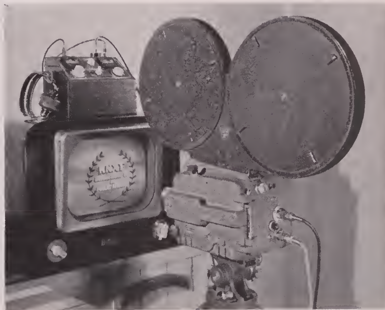
FIG. 3—Another Parrish adaptation. Here the Cine-Voice camera has been fitted with the patented Auricon kinescope shutter and Mitchell 1200-foot external film magazine for television film recording—also known as kinescoping.
