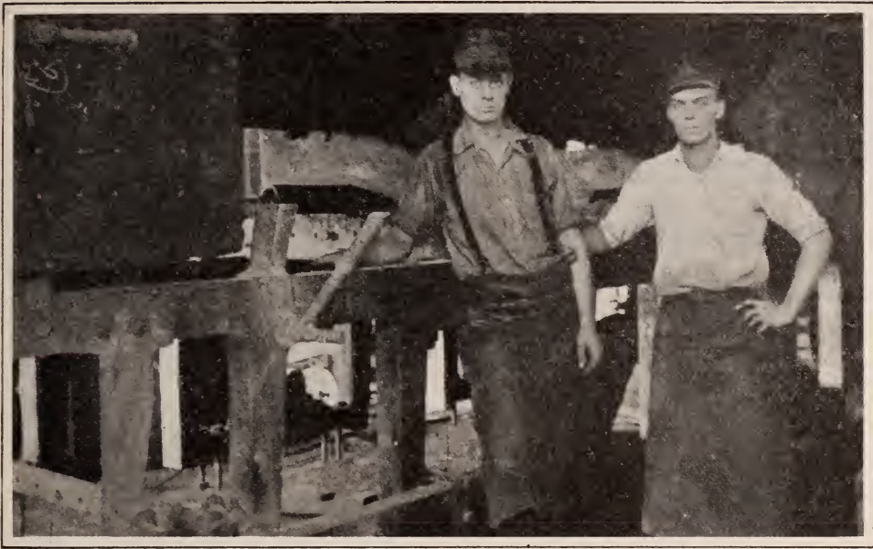
H. B. Mollohan, head blacksmith, and his helper, E. T. Miller, welding the frame of Coal and Coke Engine 54, in the Gassaway Shops
