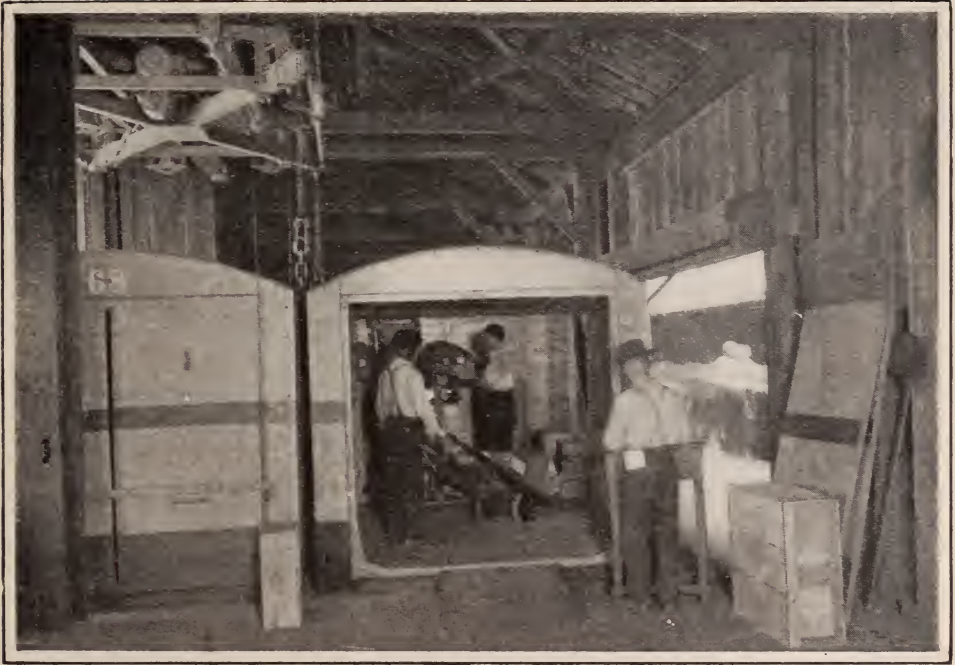
Interior of freight house; unit demountable bodies being unloaded by freight house forces; also sectional view of superstructures and electric hoist
