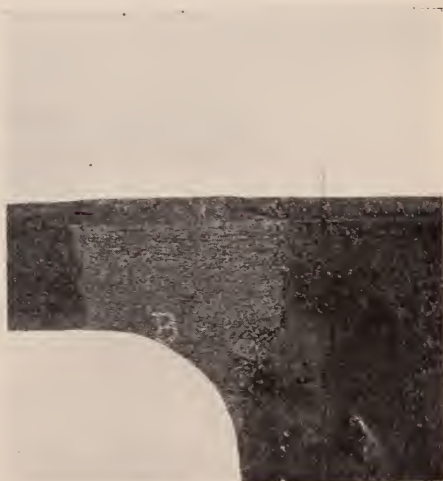
Figure 7—Electric weld in engine frame
