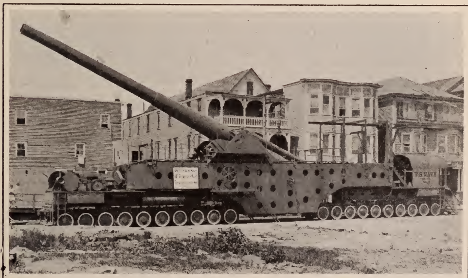
So marvelous in strength and adjustment is the recoil mechanism of this fourteen inch navy gun that it can be fired from its own trucks on railroad tracks
