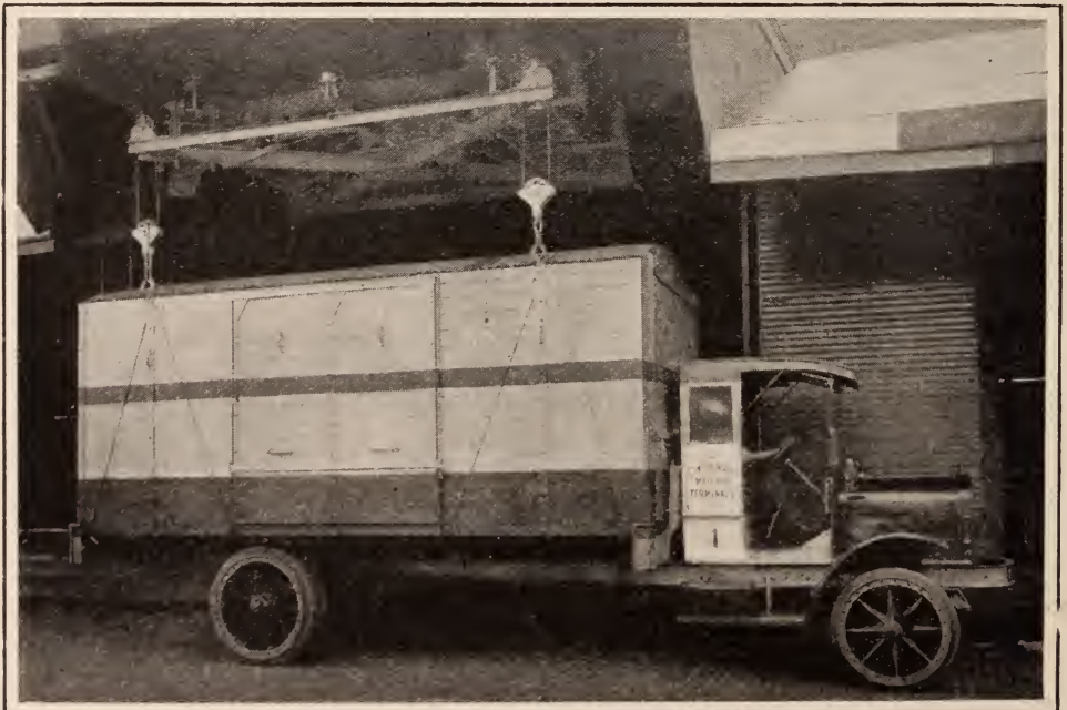
General view of freight house, entrance, superstructures, Motor Terminal Company's electric hoists, unit demountable bodies, and motor truck chassis. Body shown in position ready to be unloaded from truck chassis
