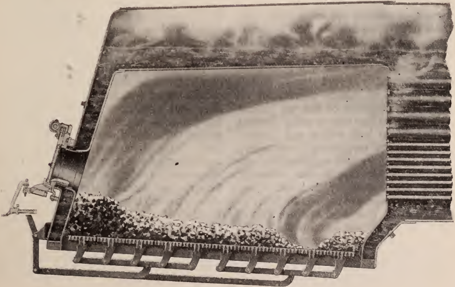
Figure 1. Hole in the Fire
