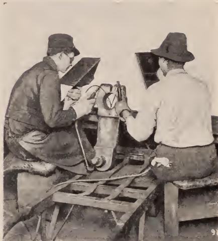
Figure 6—Building up worn fit on return crank
