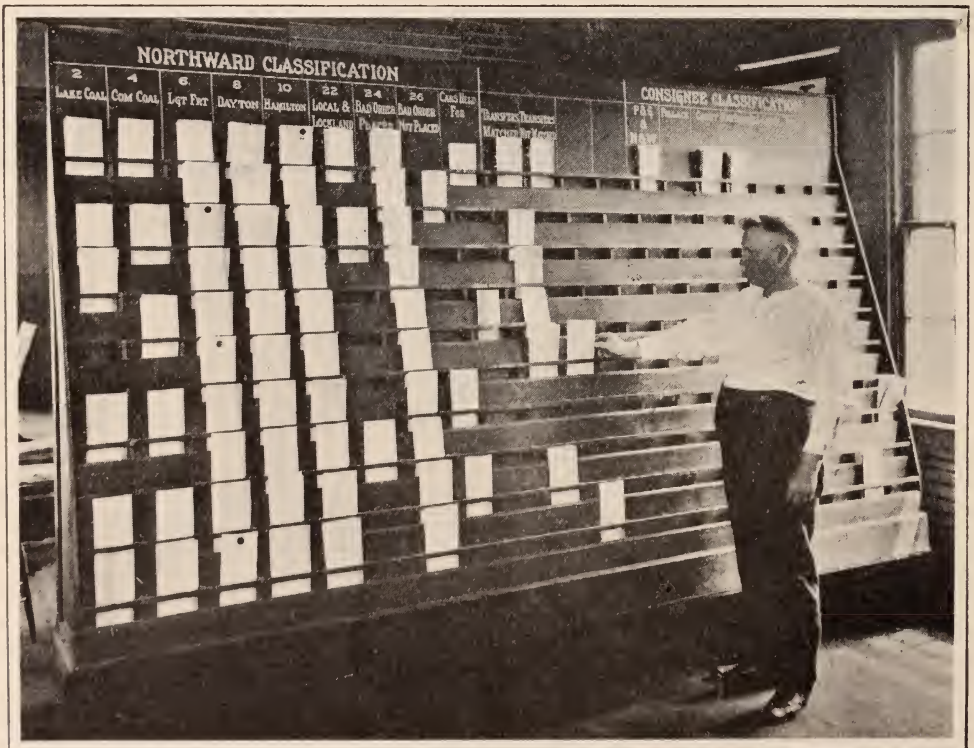
Bill rack at Elmwood, Cincinnati Terminals, northbound yard office, showing trainmaster R. B. Fitzpatrick in the act of picking out a waybill. This is the style of racks that are used at other points in Cincinnati Terminals
