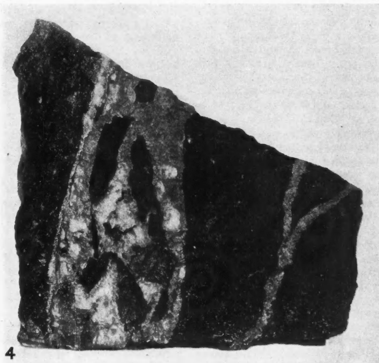
Fig. 4—Vein from Nipissing mine, showing isolated and unsupported inclusions of wall rock. In this case the fragments have a general orientation parallel to the walls, which is the more usual situation. Both this vein and the small branching vein shown contain principally niccolite, smaltite, calcite, and silver, with other minerals. The larger vein has a width of 2 inches.
