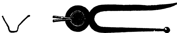
FIGS 15 AND 16. ZINC STRIP BENT INTO SHAPE AND METHOD OF PRESSING BY MEANS OF PINCERS.
