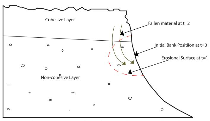
Toe erosion begins at time zero in the weaker non-cohesive layer and partially erodes a small lower portion of the cohesive layer. Erosion continues until time 1. Immediately following the removal of the non-cohesive layer, material from the cohesive layer falls at time 2. The process then begins again.
