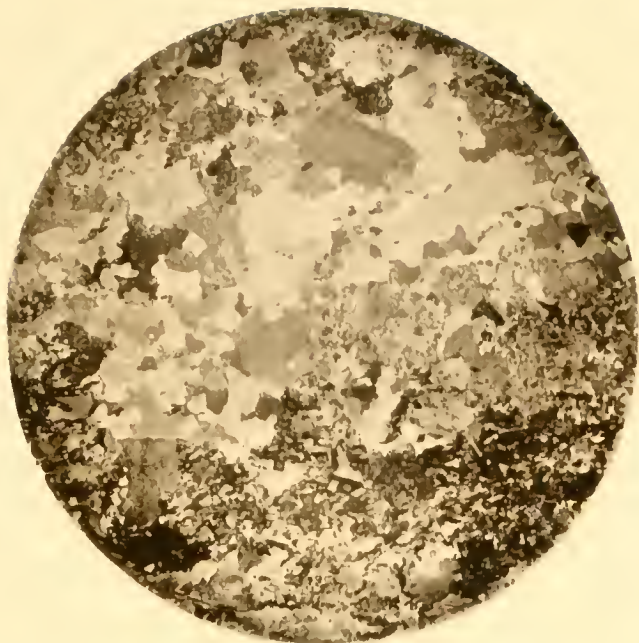
FIG. 1.—PHOTOMICROGRAPH OF GRANITE, PORT DEPOSIT. (MAGNIFIED TEN DIAMETERS.)
