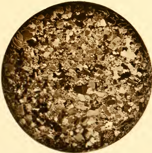
FIG. 2.—PHOTOMICROGRAPH OF GNEISS, BALTIMORE. (MAGNIFIED TEN DIAMETERS.)
