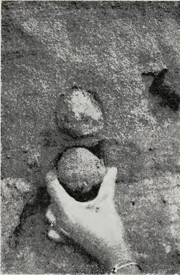
FIGURE 4. Typical Clay Ball in Stratified Sand under Valderan Till, Two Rivers, Wisconsin.
