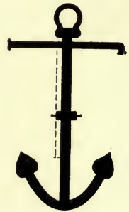
ADMIRALTY PATTERN ANCHOR WITH IRON STOCK.
