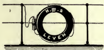
AN ORDINARY LIFEBOUY FITTED WITH HOLMES' LIGHT.
