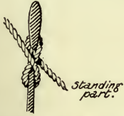
TO SECURE A ROPE ROUND A RELAYING PIN.
