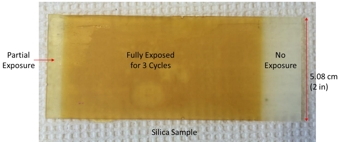
Figure 19. Color Change and Exposure Comparisons for SiO 2 Sample after Partial Exposure, 3 Cycles of Exposure and No Exposure to UV Light.
