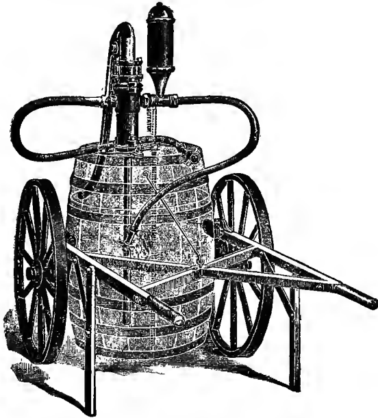
FIG. 302.—Barrel Outfit Complete with Wheels.
