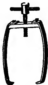
FIG. 193.—Cheap Press for heading-up Apple-Barrels.
