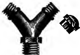
FIG. 300.—Y-Fixture for Vermorel Nozzles.
