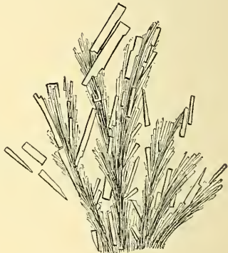
Detailed drawing showing the feather-like grouping of augite and feldspar. Magnified 100 times.
