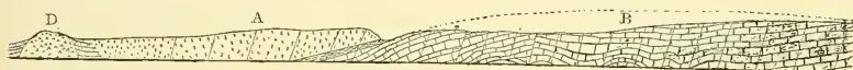
Fig. 1. Section across the Austin-New Braunfels unconformity, Travis county, Texas, showing disturbances at close of Upper (A) and lower Cretaceous (B), and unconformity between these systems. Basaltic extrusion (Pilot Knob) at D.
