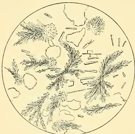
Feather-augite in basalt from Mokuaweoweo. Magnified 60 times.
