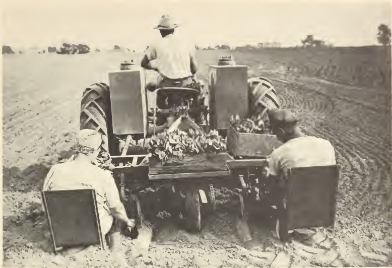
Figure 9.--Power-drawn transplanting machine.
