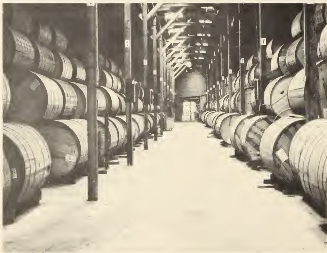
Figure 39.--Flue-cured tobacco in storage. Overhead center line of skylights are for inspection of redried hogshead tobacco.
