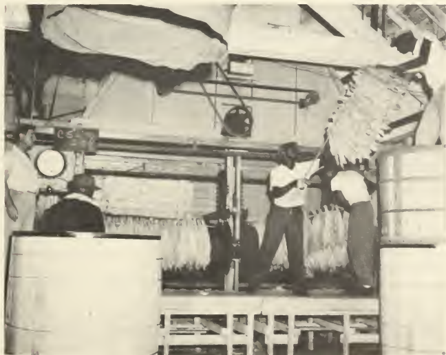
Figure 37.--Flue-cured tobacco being placed into hogs-heads as it comes from the redrying machine.
