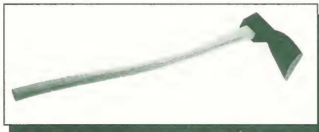
Figure 79—Using an adz safely requires that the adz has a razor-sharp edge and that the worker use the utmost control and concentration when making the swing.
