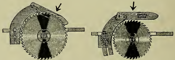
Fig. 89. Goede Saw Guard, Adjusted to Large and Small Saws.
