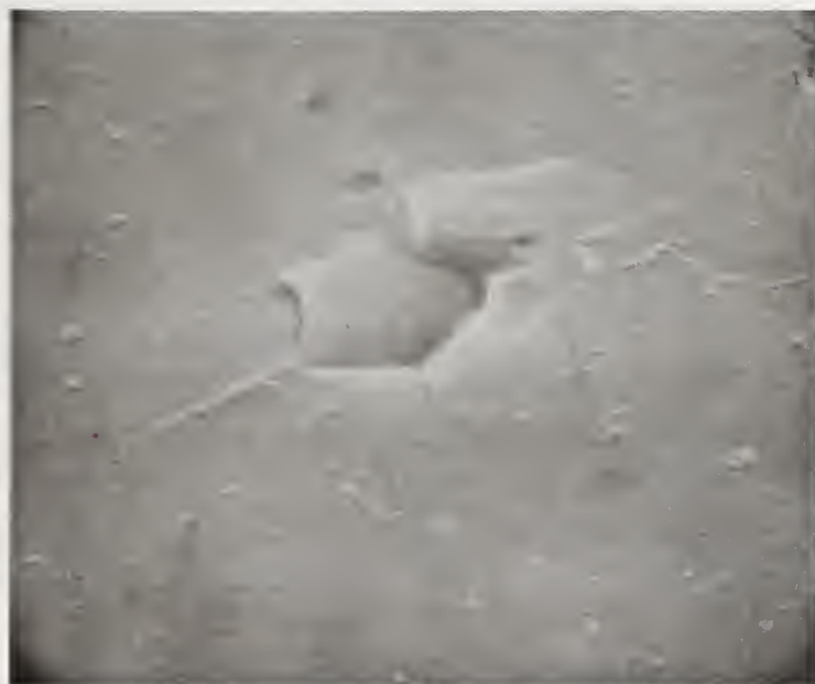
Figure 2. Scanning electron microscope photographs of cracks and holes in the silicon monoxide passivation coat near the nicrome in aluminum step of the 1509 Gate devices.
