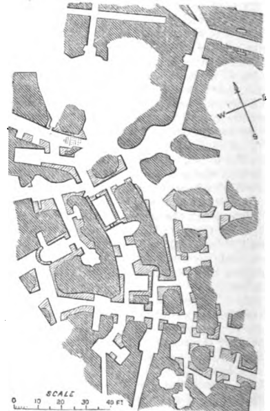
Plan of part of the Catacombs of St. Priscilla from De Rossi, showing the adaptation of an Arenaria to a Christian cemetery. The dark shading represents the tufa rock; the lighter the added masonry.
