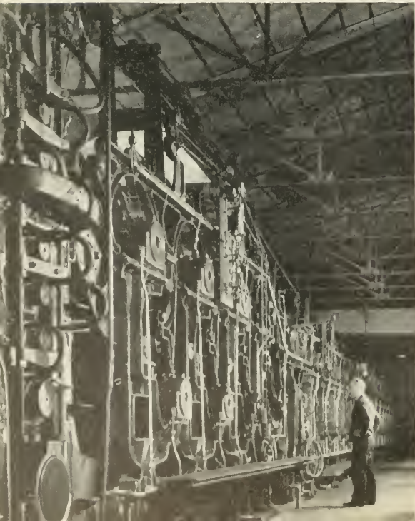
The "dry" end of a Fourdrinier machine
