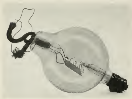
DeFOREST DETECTOR, 1908 Side view of the single plate audion
