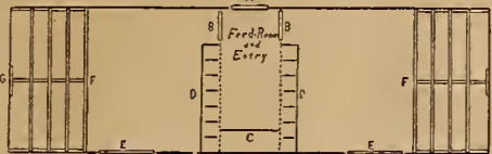
Floor plan of poultry-house. A, door; BB, inside doors; C, feed-box; DD, nests; EE, windows; FF, roosts; GG, gable windows
