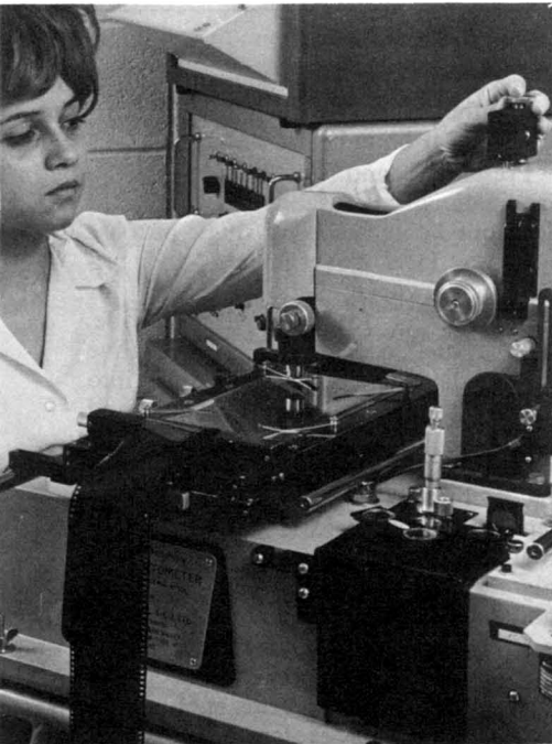
USDA technician operates machine that measures film emulsion density differences in aerial color infrared photos, a technique that may speed collection of surface data from aircraft or satellites.
